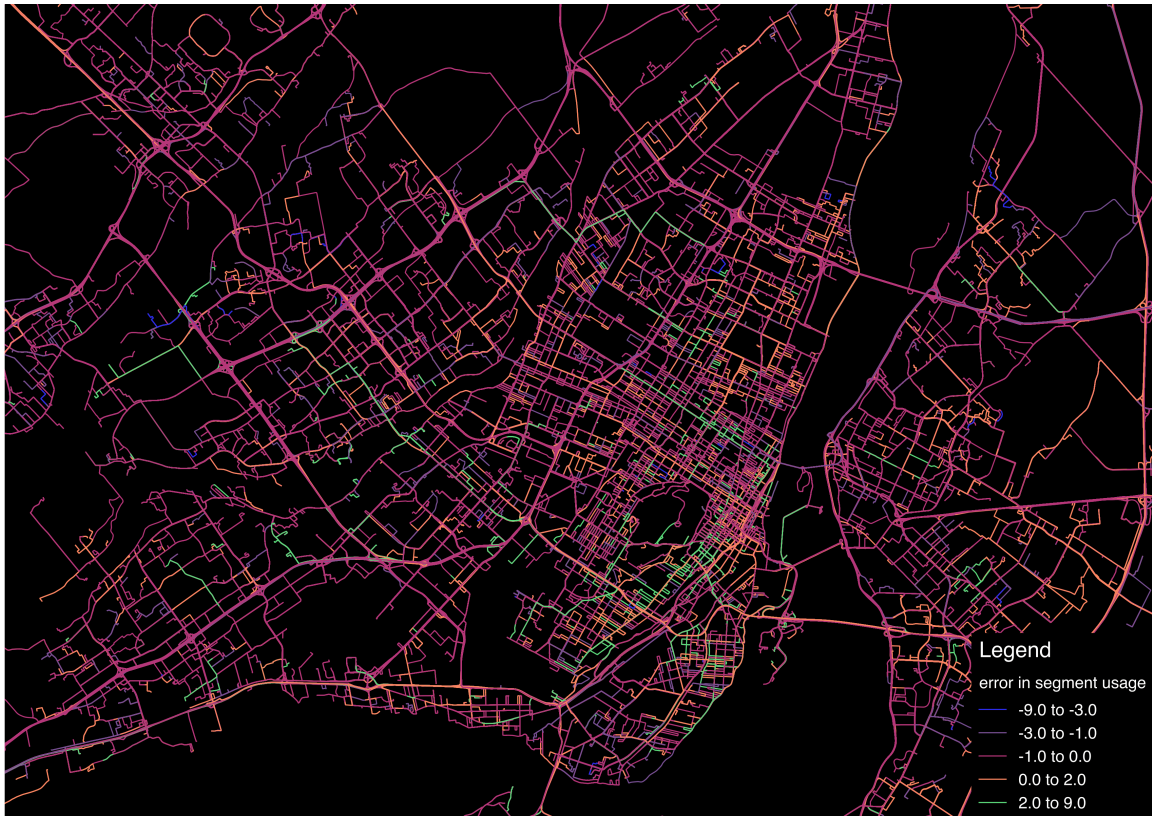
Figure 5.9: Route usage distribution of error in the simulated sequential trips of Greater Montreal Area
