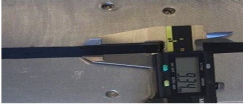
Figure 4.13. Prepreg expansion under a high compaction force (445 N)
