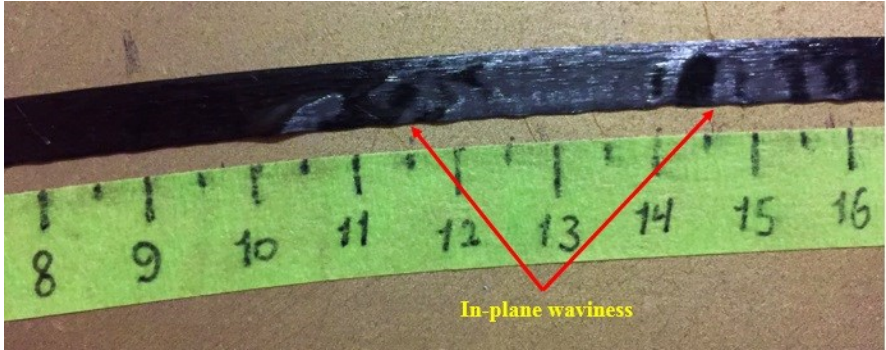
Figure 3.14. In-plane waviness as a steering defect on a steered tow
