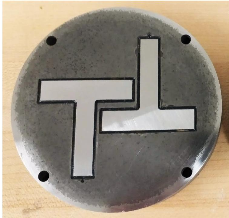
*Figure 3.6 A resin casted mounting disc.*
