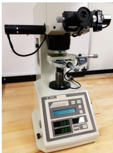
*Figure 3.17 Mitutoyo MVK-H1 micro-hardness testing machine.*
