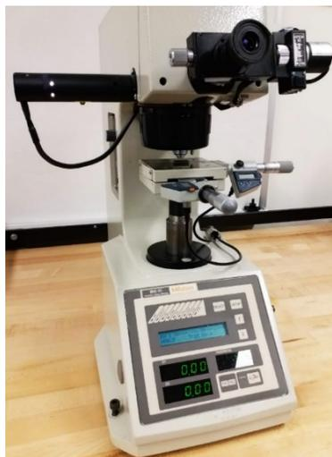
*Figure 3.17 Mitutoyo MVK-H1 micro-hardness testing machine.*
