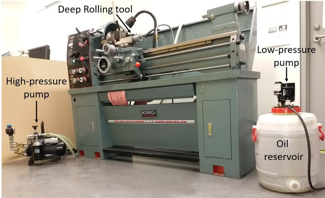
*Figure 3.7 Deep rolling setup.*
