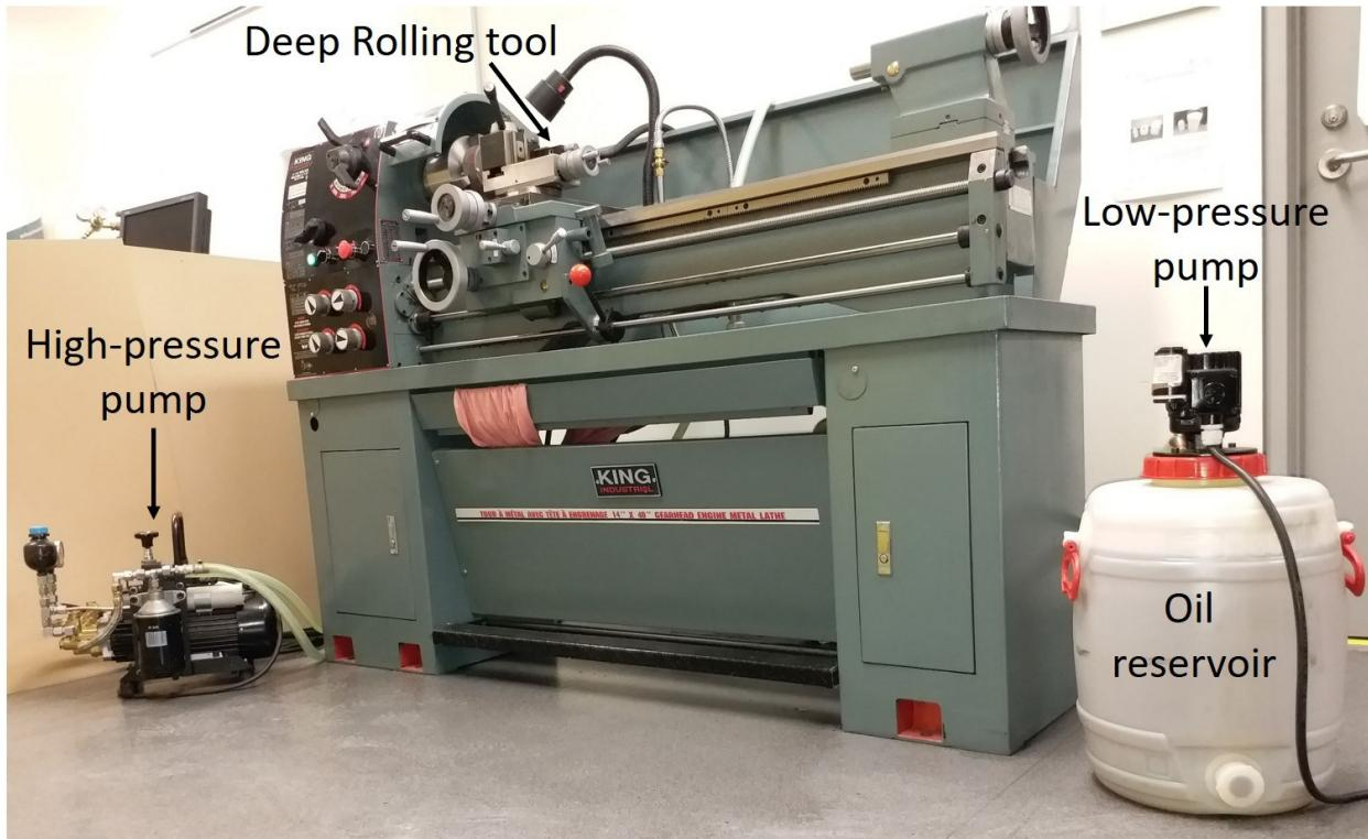
*Figure 3.7 Deep rolling setup.*
