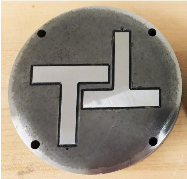
*Figure 3.6 A resin casted mounting disc.*
