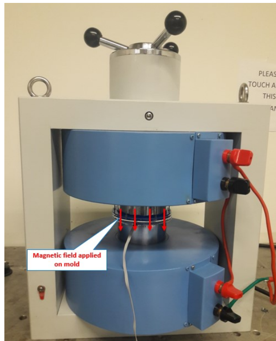
Figure 3.6 Electromagnet device used for applying magnetic field on MRE fabrication mold.
