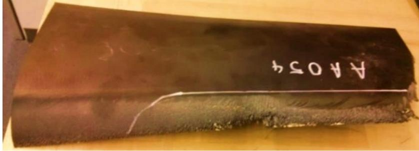
Figure 1-2 Eroded ex-service turbine blade [9].
