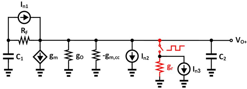
Figure 5.1: AC small-signal model, including current noise sources, of a shunt-feedback TIA with damping factor modulation by a square wave signal
