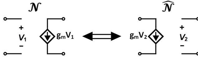
Figure 5.4: Transformation of linear voltage-controlled sources from  $\mathcal{N}$  to  $\widehat{\mathcal{N}}$  [23]
