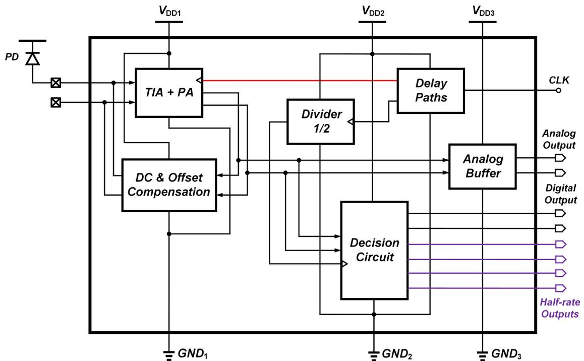
Figure 7.1: Block diagram of the designed receiver chip including the modulated damping shunt-feedback TIA and Cherry-Hooper post-amplifier, a DC/Offset compensation, an analog buffer and a decision circuit
