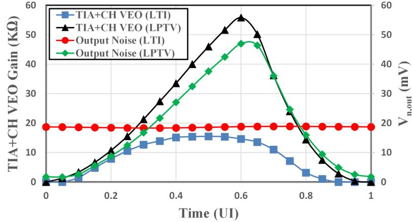
Figure 6.7: VEO and output noise voltage for the LTI TIA + LTI PA and the LPTV TIA + LPTV PA in one UI
