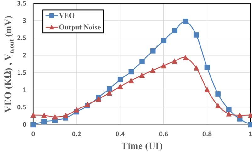
Figure 4.19: VEO and output noise voltage of the modulated damping factor TIA by a square wave in one UI
