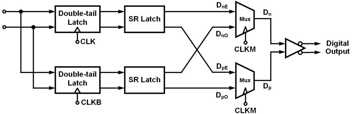
Figure 7.4: Half rate decision circuit including double-tail latches, SR-latches, 2:1 multiplexers and output buffers
