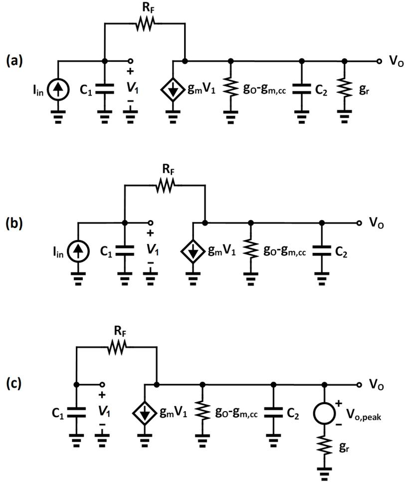
Figure 4.23: Ac small-signal model of the SF-TIA with damping factor modulation in operation mode of (a) high damping where triode-region transistor is modeled by a resistor ( $g_r$ ) (b) low damping (c) high damping where an initial dc voltage ( $V_{o,peak}$ ) models the final value of the output voltage in the previous operation mode
