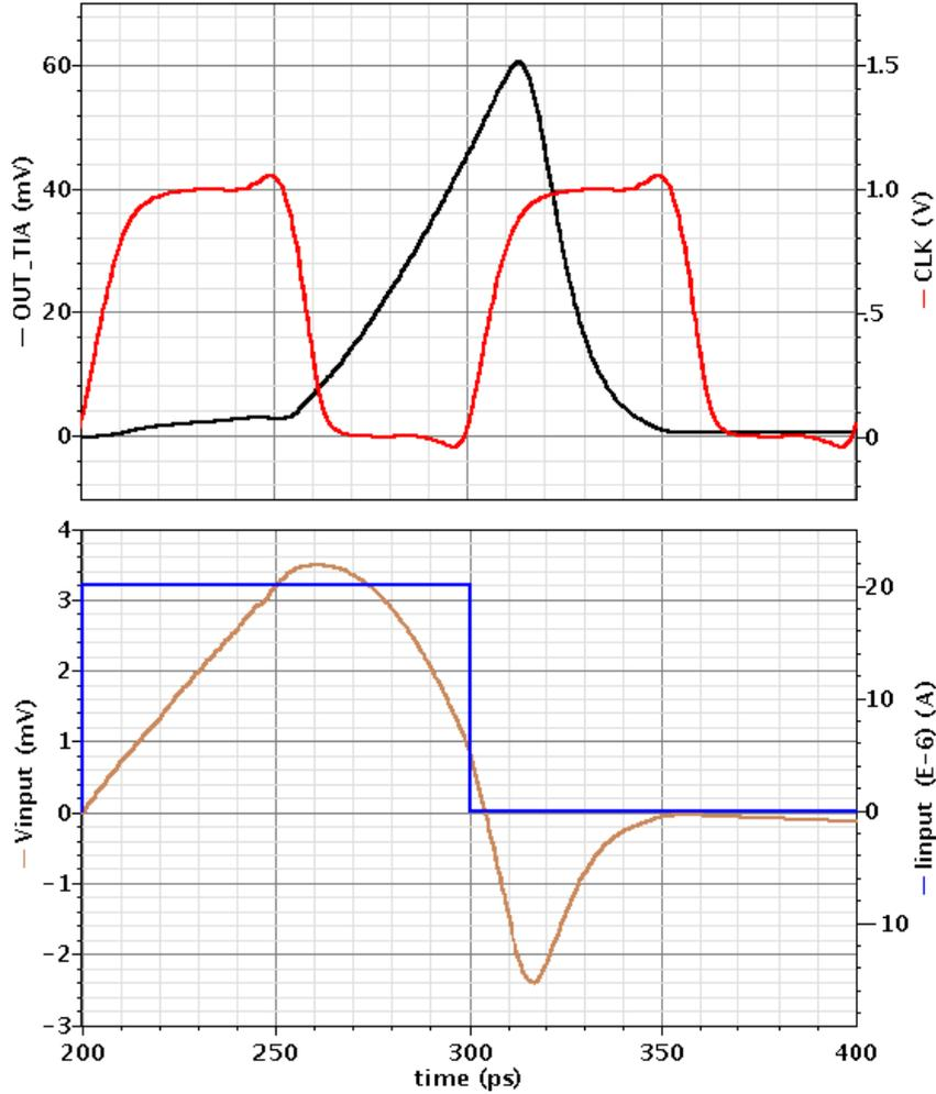
Figure 4.22: The magnified pulse response of the modulated damping shunt-feedback TIA shown in Fig. 4.20, including the modulation signal, the input pulse current and input voltage of the TIA
