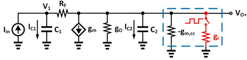
Figure 6.2: AC small-signal model of the differential half of SF-TIA
