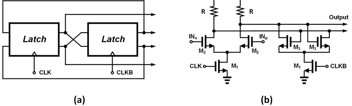
Figure 7.7: (a) Block diagram of the divider to the half-rate (b) Schematic of the CML latch including the cross-coupled transistors to regenerate at the output
