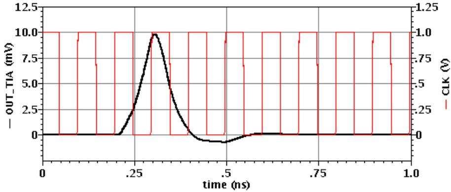
Figure 4.7: Pulse response of the shunt-feedback TIA with cross-coupled inverters at the output,  $W_1 = 30 \mu m$ ,  $W_2 = 4.5 \mu m$ ,  $R_{F1} = 100 k\Omega$ ,  $R_{F2} = 0.9 k\Omega$ ,  $t_d = 10 ps$  and  $f_{bit} = 10 Gb/s$
