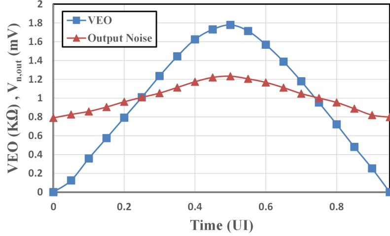
Figure 4.6: VEO and output noise voltage of shunt-feedback TIA with cross-coupled inverters at the output and  $R_F$  modulation in one UI
