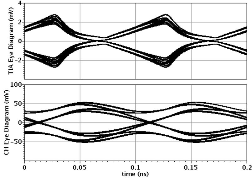
Figure 6.4: Output eye diagram of LPTV SF-TIA + LTI CH-PA,  $W_{1,2} = 30 \mu\text{m}$ ,  $W_{X1} = 11 \mu\text{m}$ ,  $W_{X2} = 4.5 \mu\text{m}$ ,  $W_{r1} = 20 \mu\text{m}$ ,  $R_{F1,2} = 1.4 \text{ k}\Omega$  and  $f_{bit} = 10 \text{ Gb/s}$
