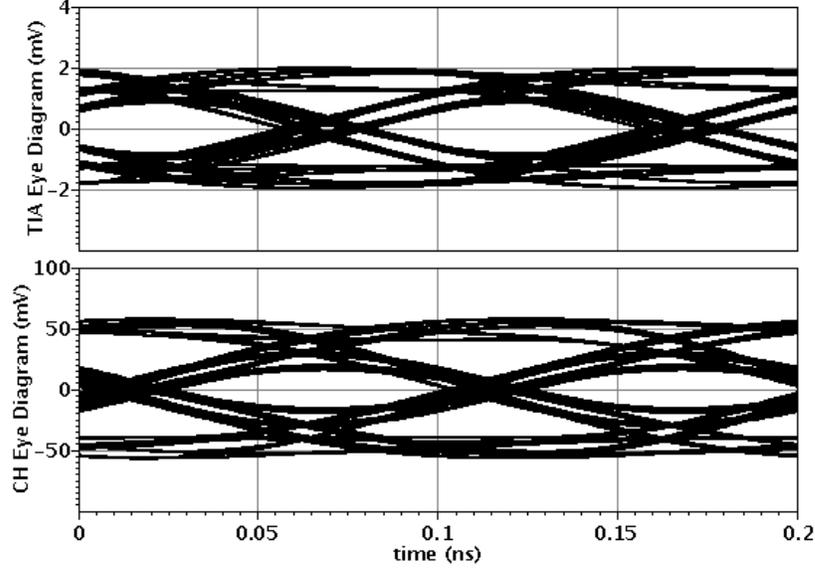
Figure 6.3: Output eye diagram of LTI SF-TIA + LTI CH-PA,  $W_{1,2} = 30 \mu m$ ,  $W_{X1,2} = 4.5 \mu m$ ,  $R_{F1,2} = 1.4 k\Omega$  and  $f_{bit} = 10 Gb/s$
