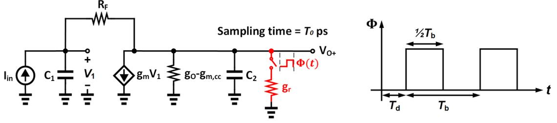
Figure 5.2: Network model ( $\mathcal{N}$ ) of the modulated damping shunt-feedback TIA with a square wave signal shown in Fig. 5.1
