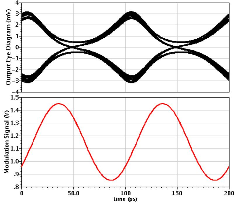
Figure 4.11: Output eye diagram of the shunt-feedback TIA with transconductance modulation by a *sin* wave signal at the output, the sinusoidal wave modulation signal,  $W_1 = 30 \mu m$ ,  $W_2 = 15 \mu m$ ,  $W_r = 4 \mu m$ ,  $R_F = 1.4 k\Omega$ ,  $A = 0.3 V$ ,  $B = 1.15 V$ ,  $\phi_{start} = 310^\circ$  and  $f_{bit} = 10 Gb/s$
