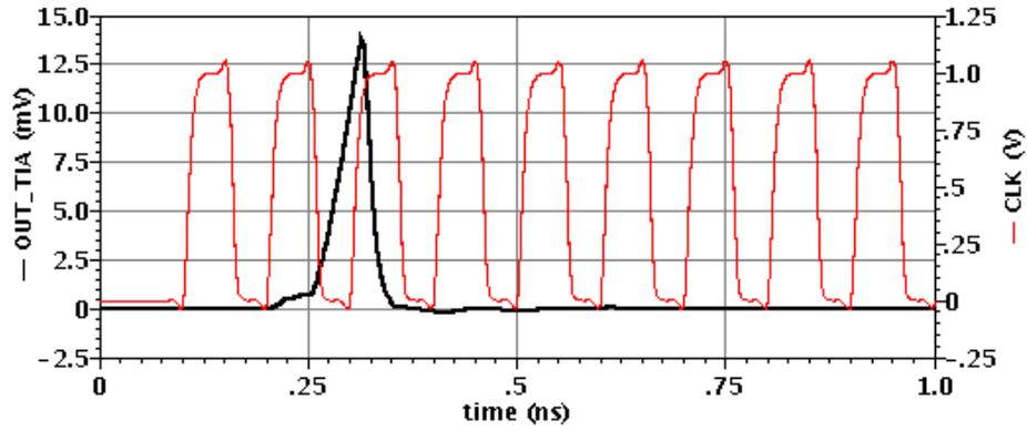
Figure 4.20: Pulse response of the shunt-feedback TIA with transconductance modulation by a rail-to-rail square wave signal at the output, the rail-to-rail square wave modulation signal,  $W_1 = 30 \mu m$ ,  $W_2 = 11 \mu m$ ,  $W_r = 20 \mu m$ ,  $R_F = 1.4 k\Omega$ ,  $t_d = 5 ps$  and  $f_{bit} = 10 Gb/s$
