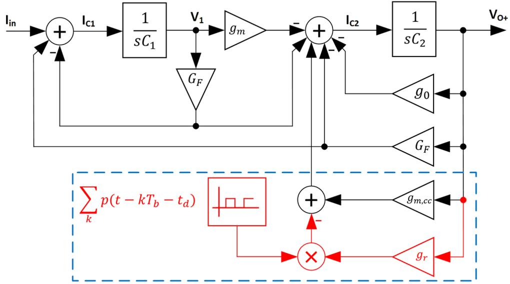
Figure 4.16: SIMULINK model of the shunt-feedback TIA with transconductance modulation by a rail-to-rail square wave signal at the output, shown in Fig. 4.15
