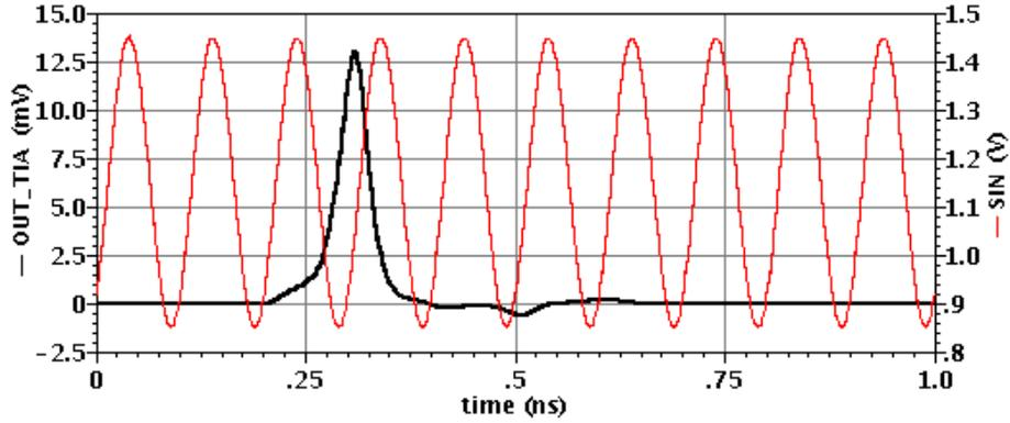
Figure 4.13: Pulse response of the shunt-feedback TIA with transconductance modulation by a sin wave signal at the output, the sinusoidal wave modulation signal,  $W_1 = 30 \mu m$ ,  $W_2 = 15 \mu m$ ,  $W_r = 4 \mu m$ ,  $R_F = 1.4 k\Omega$ ,  $A = 0.3 V$ ,  $B = 1.15 V$ ,  $\phi_{start} = 310^\circ$  and  $f_{bit} = 10 Gb/s$
