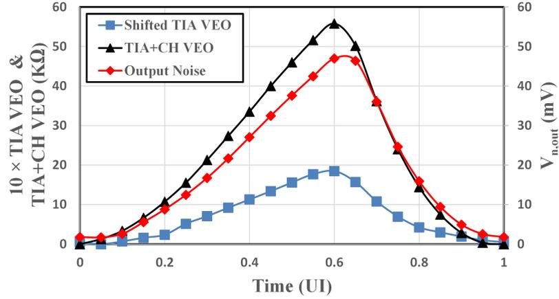
Figure 6.6: VEO, shifted VEO of the TIA and output noise voltage for the LPTV TIA + LPTV PA in one UI
