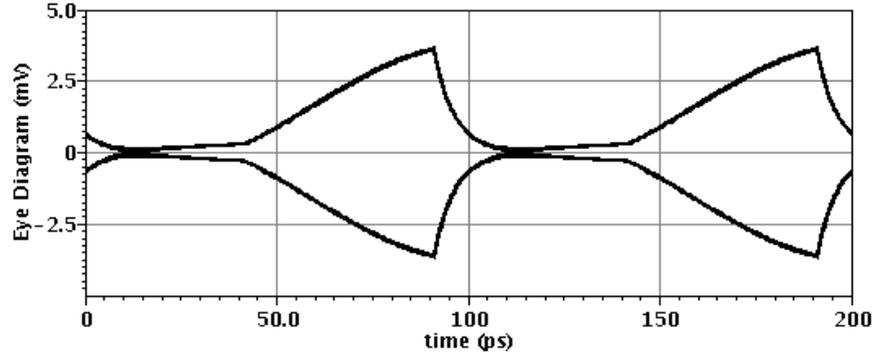
Figure 5.3: Output eye diagram of the network model ( $\mathcal{N}$ ) shown in Fig. 5.2,  $C_1 = 230 \text{ fF}$ ,  $C_2 = 50 \text{ fF}$ ,  $R_F = 1.4 \text{ k}\Omega$ ,  $g_m = 22 \text{ m}\mathcal{U}$ ,  $g_o - g_{m,cc} = -1 \text{ m}\mathcal{U}$ ,  $g_r = 10 \text{ m}\mathcal{U}$ ,  $T_b = 100 \text{ ps}$ ,  $T_d = 9 \text{ ps}$  and  $f_{bit} = 10 \text{ Gb/s}$
