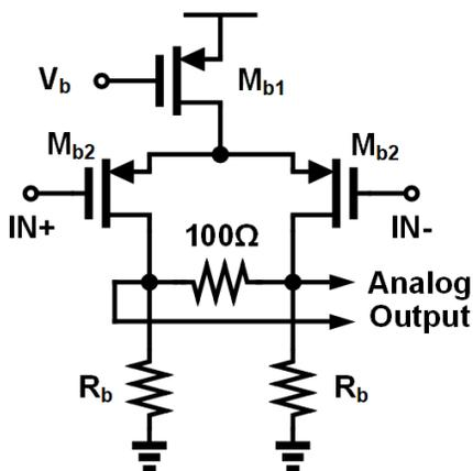
Figure 7.3: Schematic of the CML analog buffer to drive  $100 \Omega$  resistance load
