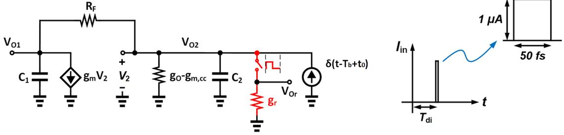
Figure 5.5: Adjoint network model ( $\hat{\mathcal{N}}$ ) of the modulated damping shunt-feedback TIA,  $C_1 = 230 \text{ fF}$ ,  $C_2 = 50 \text{ fF}$ ,  $R_F = 1.4 \text{ k}\Omega$ ,  $g_m = 22 \text{ m}\mathcal{U}$ ,  $g_o - g_{m,cc} = -1 \text{ m}\mathcal{U}$ ,  $g_r = 10 \text{ m}\mathcal{U}$  and  $T_{di} = T_b - T_0 = 9 \text{ ps}$
