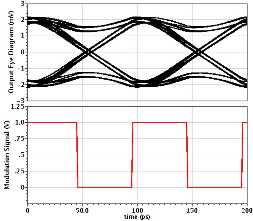
Figure 4.5: Output eye diagram of the shunt-feedback TIA with cross-coupled inverters at the output and  $R_F$  modulation, the rail-to-rail square wave modulation signal,  $W_1 = 30 \mu m$ ,  $W_2 = 4.5 \mu m$ ,  $R_{F1} = 100 k\Omega$ ,  $R_{F2} = 0.9 k\Omega$ ,  $t_d = 10 ps$  and  $f_{bit} = 10 Gb/s$
