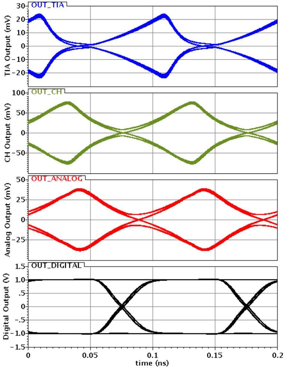
Figure 7.9: Output eye diagram of the shunt-feedback TIA, Cherry-Hooper post-amplifier, analog buffer and decision circuit
