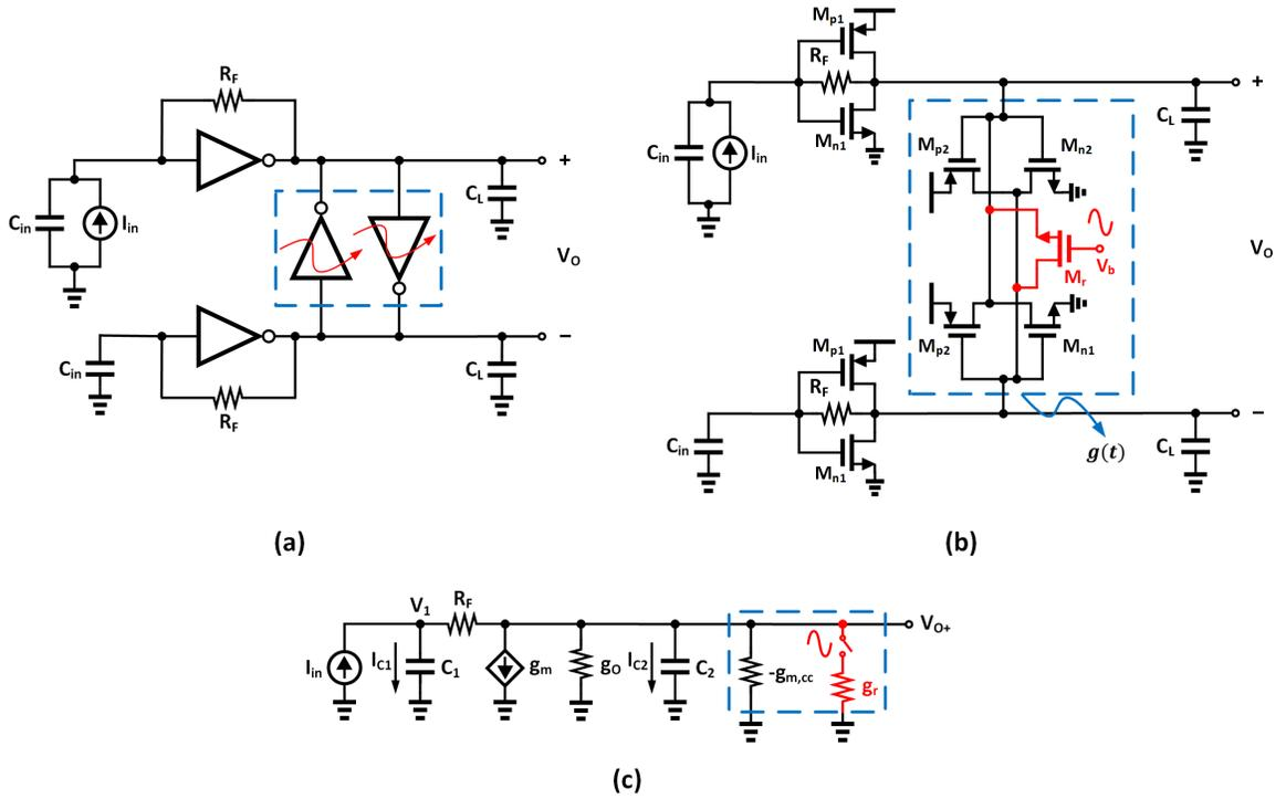
Figure 4.8: Differential shunt-feedback TIA including transconductance modulation by a *sin* wave signal at the output ( $V_b = B + A \sin(2\pi f_{bit} + \phi_{start})$ ) (a) high-level schematic (b) transistor-level schematic (c) ac small-signal model of the differential half of circuit
