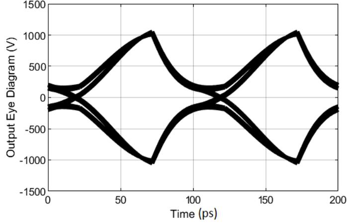
Figure 4.17: Output eye diagram of the shunt-feedback TIA model in SIMULINK with transconductance modulation by a rail-to-rail square wave signal at the output (Fig. 4.16) for input data with peak to peak amplitude of 1 A,  $g_{m,cc} = 4.4 \text{ m}\mathcal{U}$ ,  $G_F = 1 \text{ m}\mathcal{U}$ ,  $g_r = 3.3 \text{ m}\mathcal{U}$ ,  $t_d = 69 \text{ ps}$  and  $f_{bit} = 10 \text{ Gb/s}$
