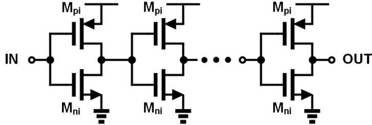
Figure 7.8: Schematic of a delay path including a number of series CMOS inverters to produce variable delays
