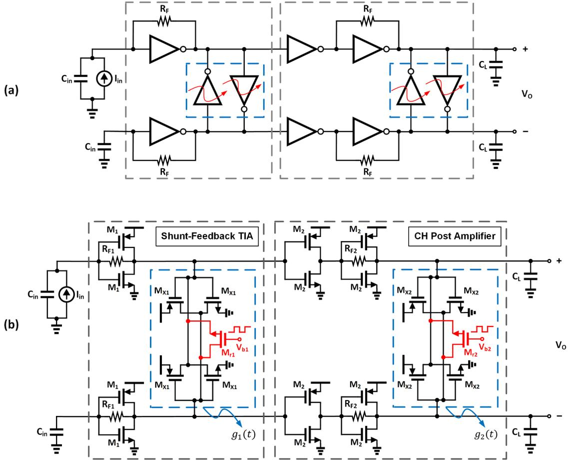
Figure 6.1: Differential shunt-feedback TIA followed by CH post-amplifier with conductance modulation at outputs (a) high-level schematic (b) transistor-level schematic. Transistors  $M_{r,1,2}$  are modulated with voltages  $V_{b1,2}$  synchronously with incoming data.
