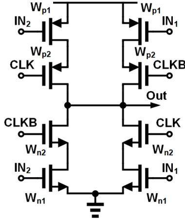
Figure 7.6: Schematic of a 2:1 multiplexer
