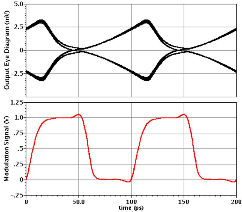
Figure 4.18: Output eye diagram of the shunt-feedback TIA with transconductance modulation by a rail-to-rail square wave signal at the output, the rail-to-rail square wave modulation signal,  $W_1 = 30 \mu m$ ,  $W_2 = 11 \mu m$ ,  $W_r = 20 \mu m$ ,  $R_F = 1.4 k\Omega$ ,  $t_d = 5 ps$  and  $f_{bit} = 10 Gb/s$
