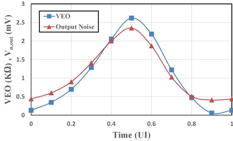
Figure 4.12: VEO and output noise voltage of the modulated damping factor TIA by a *sin* wave in one UI
