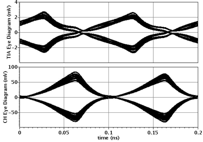
Figure 6.5: Output eye diagram of LPTV SF-TIA + LPTV CH-PA,  $W_{1,2} = 30 \mu m$ ,  $W_{X1,2} = 11 \mu m$ ,  $W_{r1,2} = 20 \mu m$ ,  $R_{F1,2} = 1.4 k\Omega$  and  $f_{bit} = 10 Gb/s$
