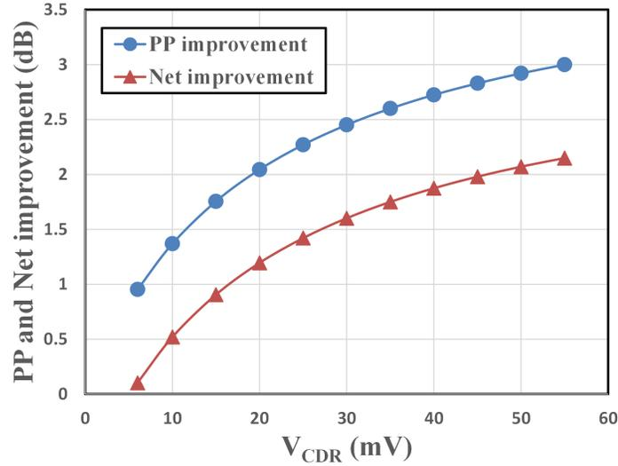
Figure 4.14: Power Penalty (PP) and net performance improvement of the TIA with damping factor modulation with *sin* wave compared to the TIA with cross-coupled inverters at the output over a range of minimum clock-and-data recovery voltage swing
