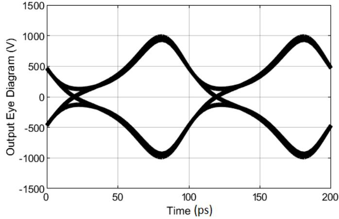
Figure 4.10: Output eye diagram of the shunt-feedback TIA model in SIMULINK with transconductance modulation by a *sin* wave signal at the output (Fig. 4.9) for input data with peak to peak amplitude of 1 A,  $g_{m,cc} = 1\text{U}$ ,  $G_F = 1\text{ mU}$ ,  $g_r = 1\text{ mU}$ ,  $A = 3$ ,  $B = -0.2$ ,  $\phi_{start} = 0.6\text{ rad}$  and  $f_{bit} = 10\text{ Gb/s}$
