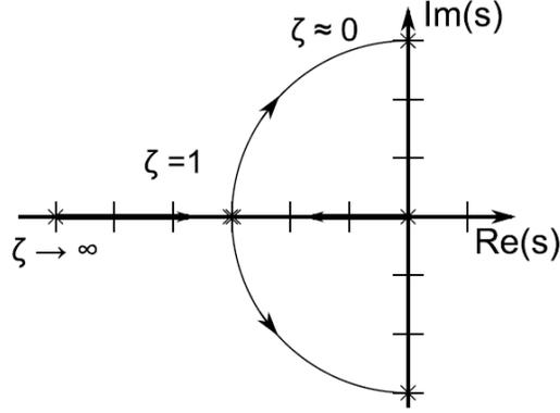
Figure 4.24: Location of the poles of a 2<sup>nd</sup>-order system as the damping factor  $\zeta$  goes from  $\infty$  to 0 [22]
