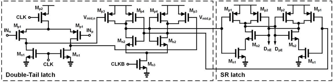
Figure 7.5: Schematic of a double-tail latch followed by a SR-latch
