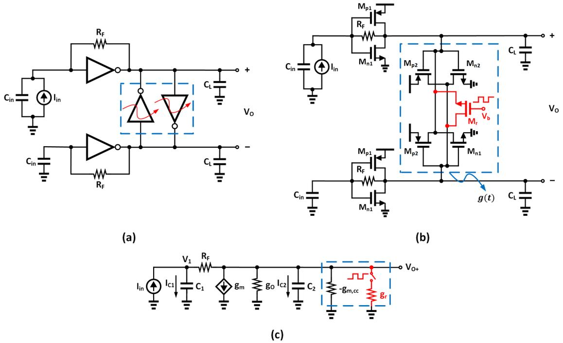
Figure 4.15: Differential shunt-feedback TIA including transconductance modulation by a rail-to-rail square wave signal at the output ( $V_b = V_{DD} \sum p(t - kT_b - t_d)$ ) (a) high-level schematic (b) transistor-level schematic (c) ac small-signal model of the differential half of circuit
