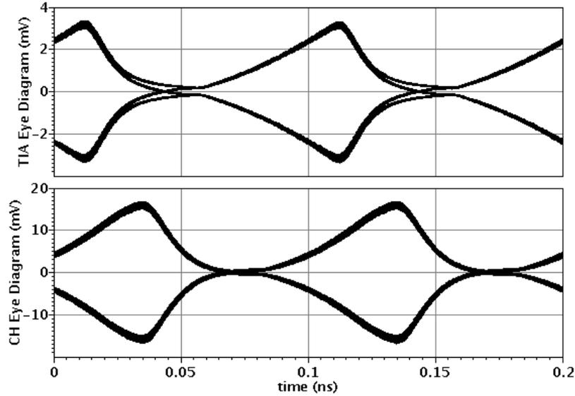
Figure 6.8: Output of the low power LPTV SF-TIA + LPTV CH-PA system,  $W_1 = 30 \mu\text{m}$ ,  $W_2 = 8 \mu\text{m}$ ,  $W_{X1} = 11 \mu\text{m}$ ,  $W_{X2} = 4 \mu\text{m}$ ,  $W_{r1} = 20 \mu\text{m}$ ,  $W_{r2} = 8 \mu\text{m}$ ,  $R_{F1} = 1.4 \text{ k}\Omega$ ,  $R_{F2} = 0.8 \text{ k}\Omega$  and  $f_{bit} = 10 \text{ Gb/s}$
