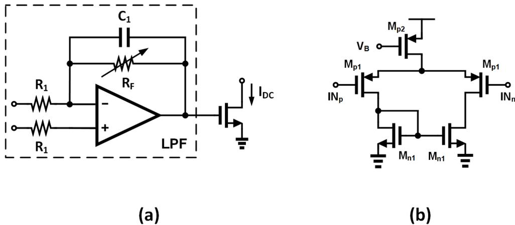
Figure 7.2: Schematic of (a) DC/offset compensation including an active low-pass filter followed by a current source (b) the single-ended differential amplifier
