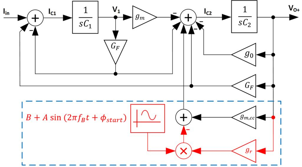
Figure 4.9: SIMULINK model of the shunt-feedback TIA with transconductance modulation by a *sin* wave signal at the output, shown in Fig. 4.8
