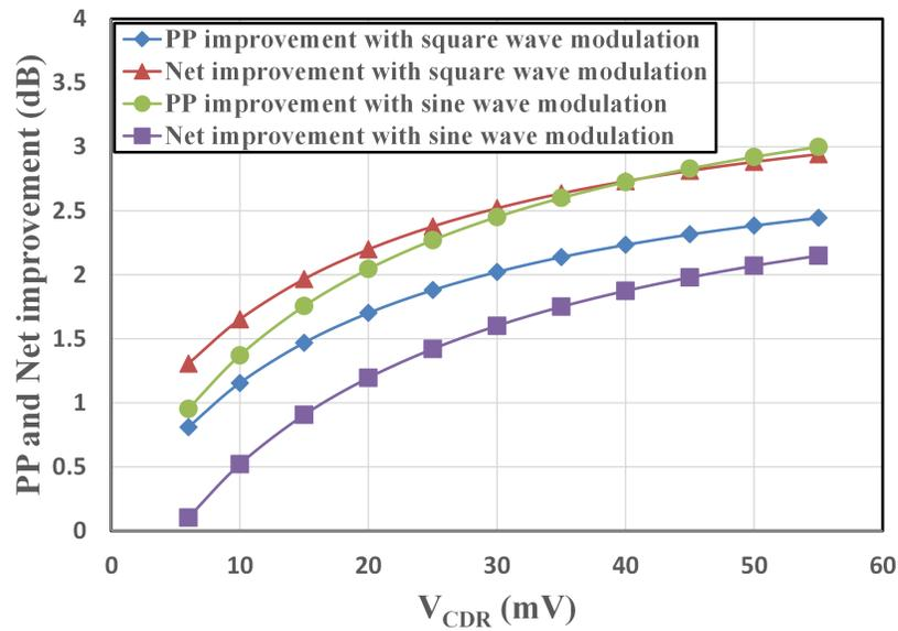
Figure 4.21: Power Penalty (PP) and net performance improvement of the TIA with damping factor modulation by *sin* and rail-to-rail square waves compared to the TIA with cross-coupled inverters at the output over a range of minimum clock-and-data recovery voltage swing
