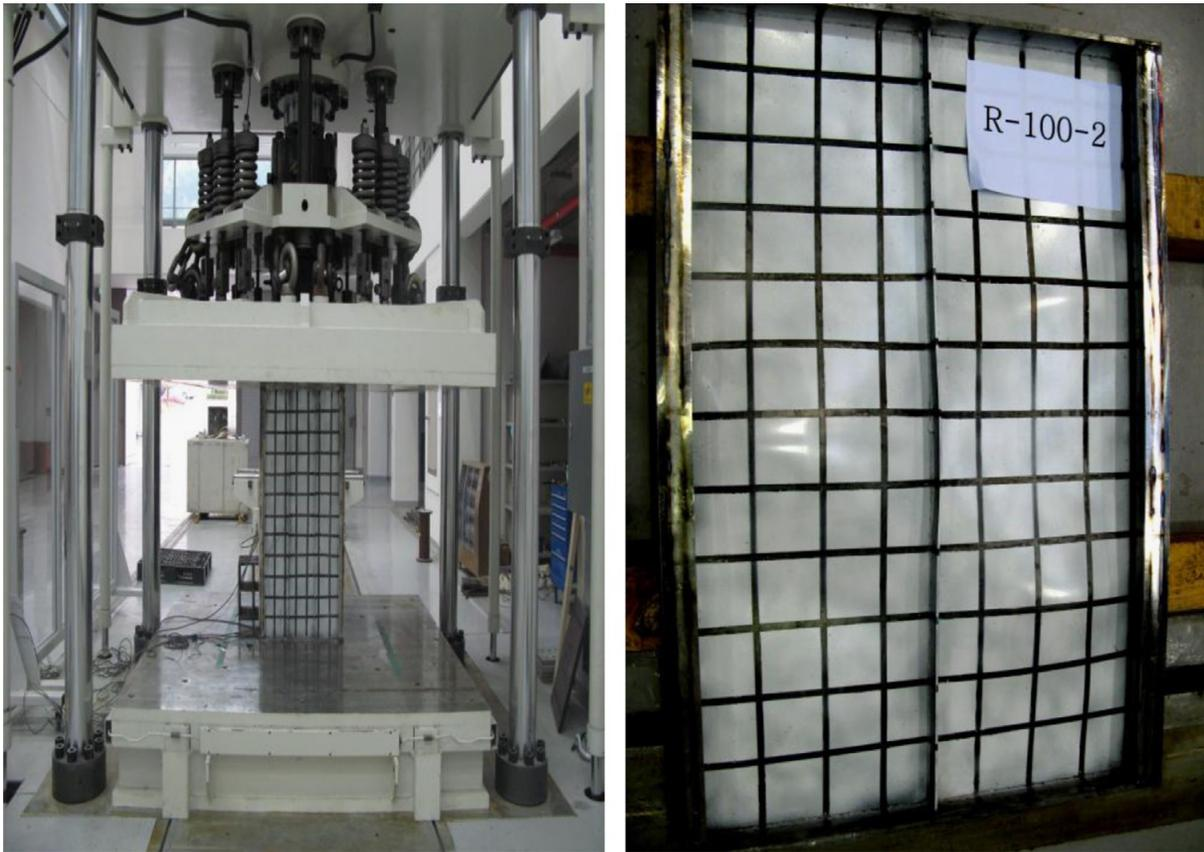
Fig. 2.12: Test setup and deformed shape of the stiffened plate specimen (Kwon, 2014)
