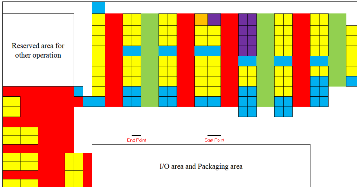
Figure 1: Warehouse Layout (Lane Type: Green indicates wide aisle, Red indicates Narrow/ Congested aisle; Rack Type: Blue: 1-Tier, Yellow: 2-Tiers, Orange: 3-Tiers, Purple: 4-Tiers)
