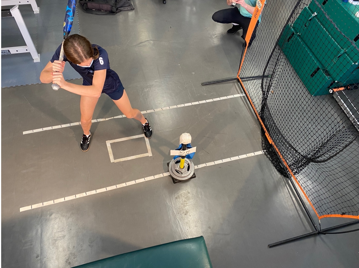
Figure 8 . A picture of the data measurement set-up We can see distance markers on the floor to facilitate the calibration of the Kinovea software. We can see a participant holding his own bat just before he swings towards a ball into a net from a tee.
