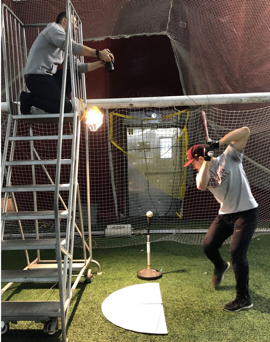
Figure 5. A picture of the data measurement set-up. We can see distance markers on the floor to facilitate the calibration of the Kinovea software. We can see a participant holding his own bat just before he swings towards a ball on a tee. In a ladder, I was filming using a high-speed camera the swing of the participant. Extra lights had to be added to compensate for the darkness of the indoor field to allow use to see something on the high-speed footage. The ball is batted into a net as a safety measure.
