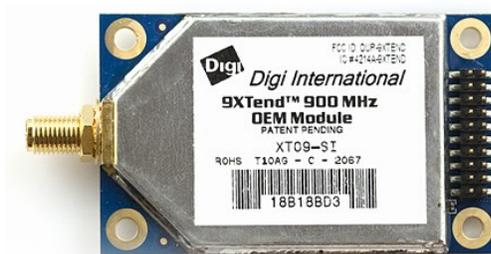
Figure 5.4: Wireless data module
