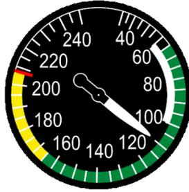
Figure 3.6: Airspeed indicator
