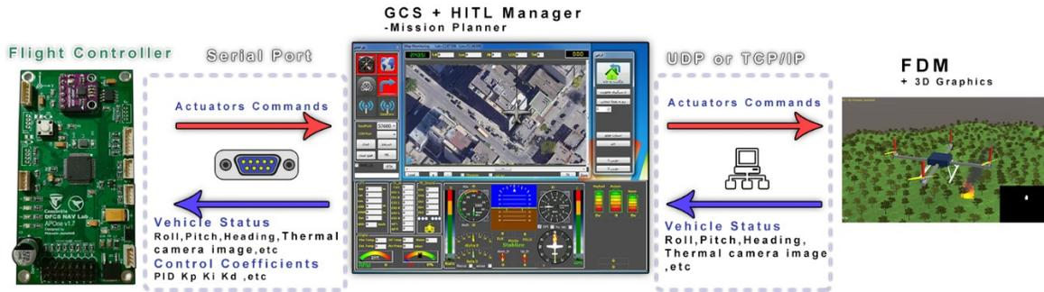
Figure 5.1: The components' connection diagram
