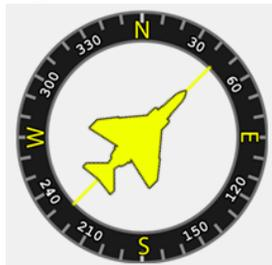
Figure 3.16: The heading indication with a 45 degree heading.
