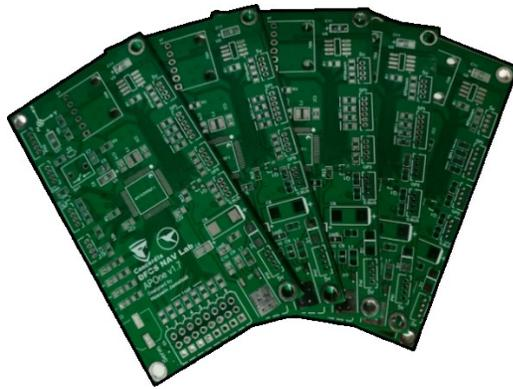
Figure 2.14: APOne v1.7 Printed board before assembly
