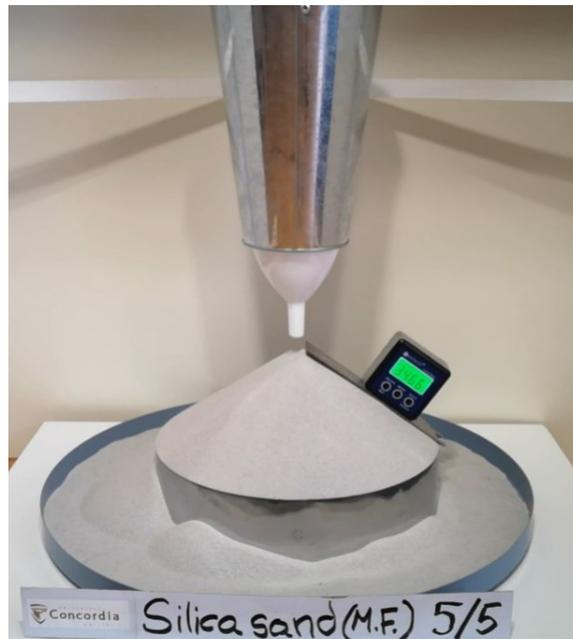
Fig. 3-7 *Fixed base and moving funnel* device after a single test on silica sand.
