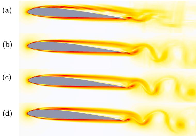
Figure 14: Contours of vorticity magnitude for the SD7003 verification case at  $Re = 10^4$  with  $p_s = 1, 2, 3$  and  $4$  at  $\alpha = 4^\circ$ .
