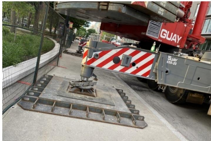
Fig. 1. Crane support system. (Photograph by Ali Nikeghbali)
