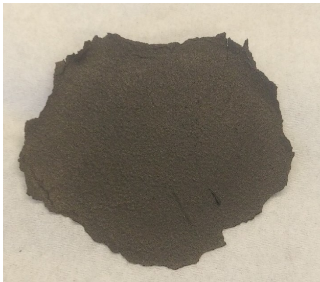
Figure 6-1: A photograph of graphene oxide paper prepared by photocuring a dispersion in 1-PtOH followed by annealing, demonstrating its substantial size and uniformity.
