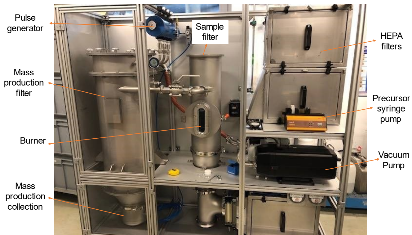
Figure 2-5: FSP setup at Concordia University- first in Canada.
