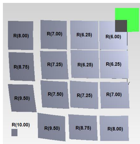
Figure 49: Radius of curvature of reflector design – iteration 1
