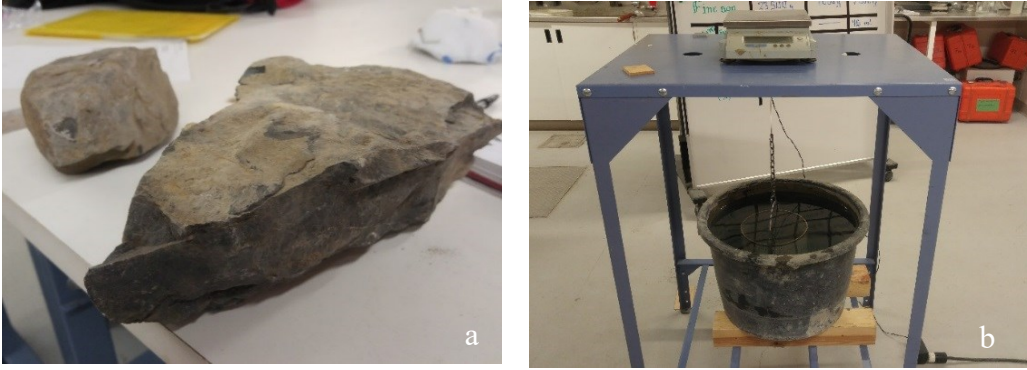
Figure 4.23: a) Limestone masonry samples collected from the field near the building prepared for density test b) Measurement of the weight in water using a chain hooked to the weight balance.
