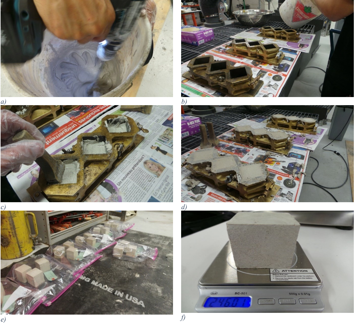
Figure 4.21: a) Mixing the mortar using a mechanical turbine b) ASTM certified molds c) Tapping the mortar at half the portion d) Finishing the surface of the mortar e) Curing f) Weight measuring.
