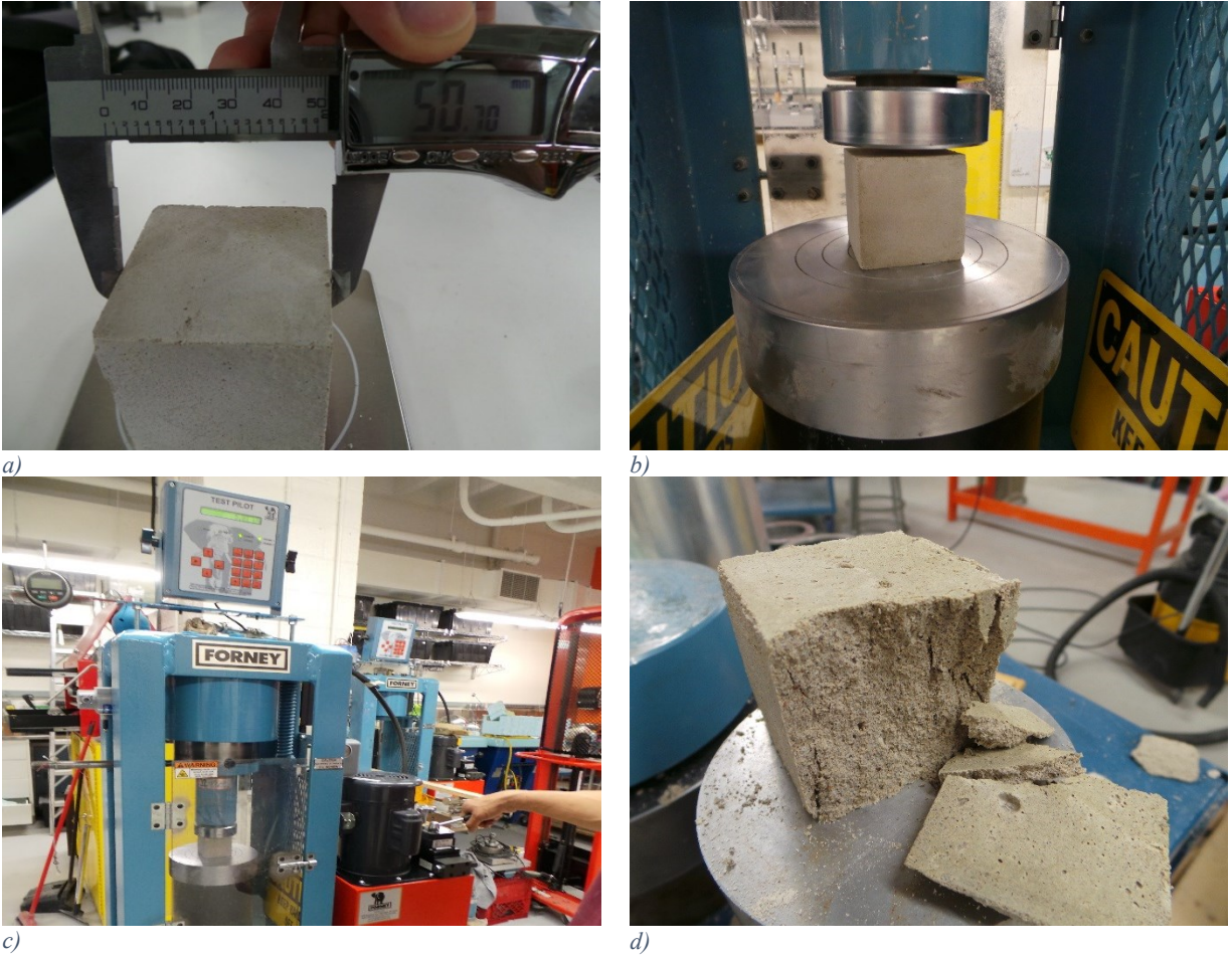
Figure 4.22: a) Measuring the dimensions b), c) Compressive strength test d) Typical failure in the mortar cubes.
