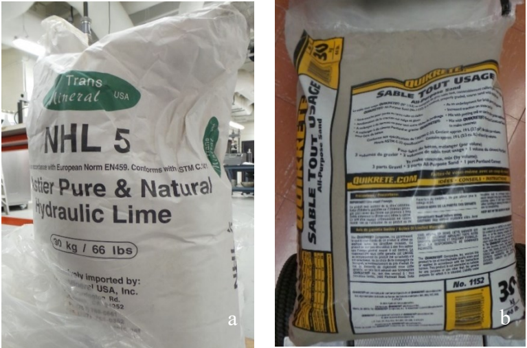
Figure 4.20: a) NHL hydraulic lime used in the mix of mortar b) Sand used in the mortar
