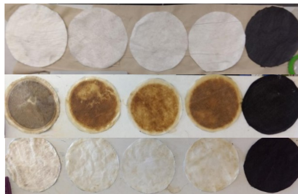
Figure 5-3: Unused, used and washed geotextiles layers (top – bottom) in the following AOS order from left to right (110 \mu\text{m} , 100 \mu\text{m} , 90 \mu\text{m} , 70 \mu\text{m} , and 65 \mu\text{m} )
