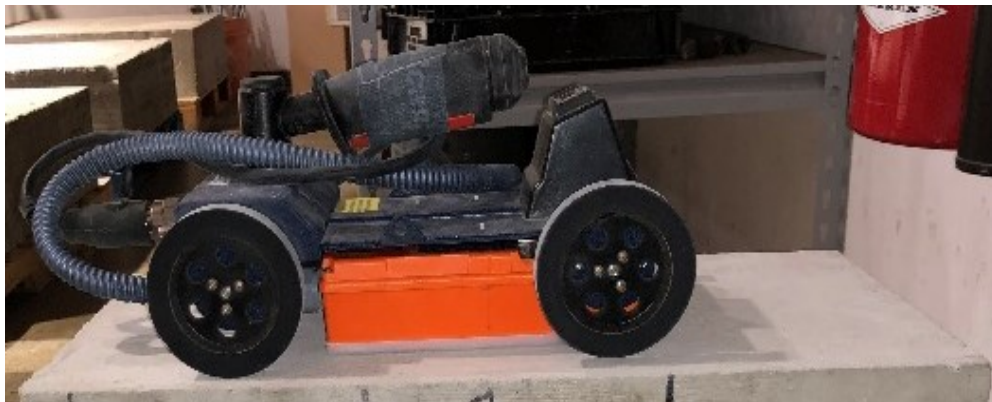
Figure 13: GPR antenna mounted on a handheld mini cart used to scan along the length of the slab
