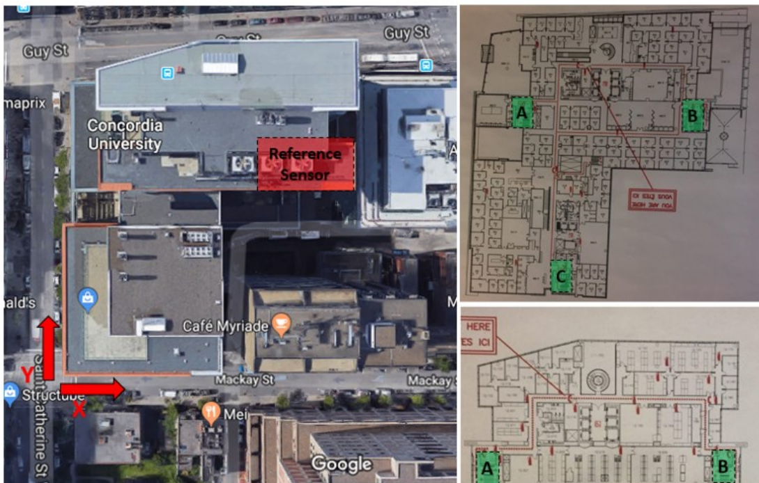
Figure 4. 3. The layout of the sensor placements for AVT over EV building (courtesy of the pictures from left to right: Google Map, Concordia university)
