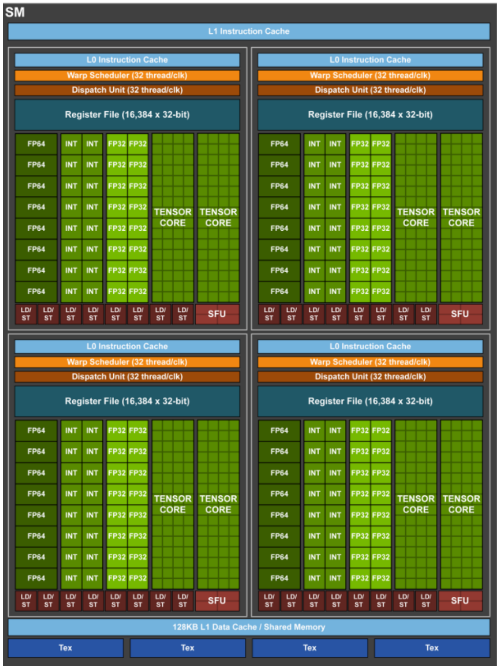
Figure 2.3: Volta GV100 Streaming multiprocessor used in Tesla V100 [41]
