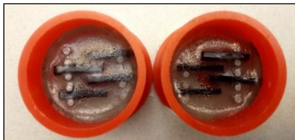
Figure 3-11 Immersed samples in the resin epoxy
