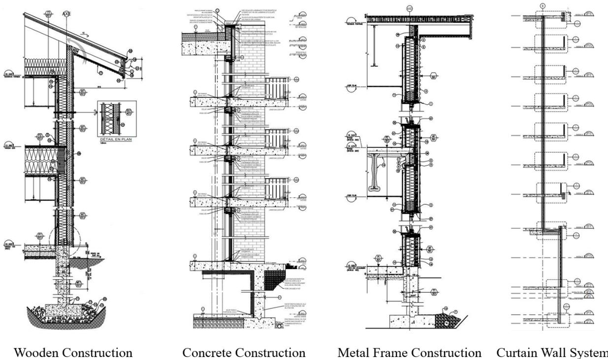
*Figure 9: Different construction types of the comparative case study buildings*
