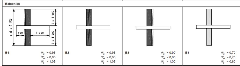
Figure 1: Default values of linear thermal bridge coefficient for balconies (ISO, 2017c)
