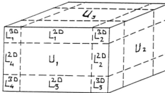
Figure 2: 1D, 2D, and 3D partitioning of the building envelope (ISO, 2017a)
