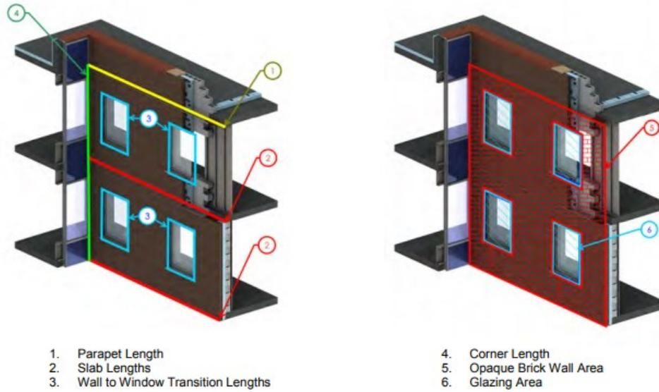
Figure 3: Building envelope area and length takeoffs (MH, 2018a)
