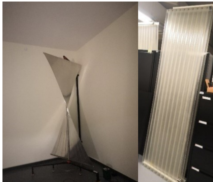
Figure 1. Steel rotating diffuser (left) and corrugated plastic hanging diffusers (right).
