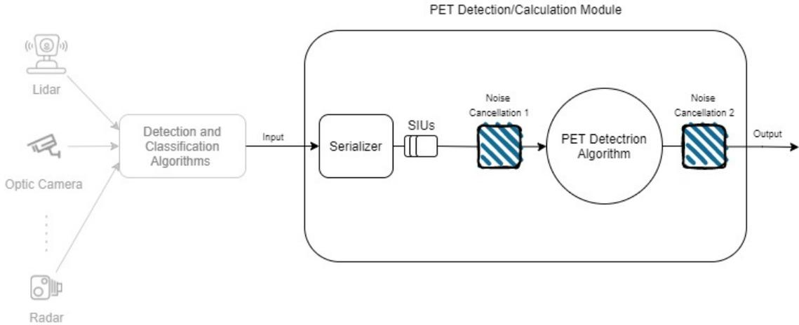
Figure 3.1: Basic PET module pipeline
