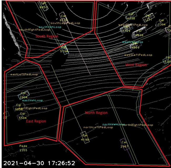
Figure 3.9: Four regions defined on BlueCity lidar image for a sensor in Edmonton, Canada
