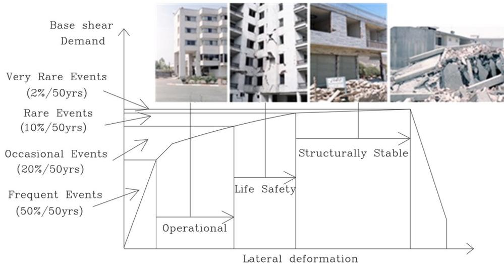
Figure 2-1. A schematic view of selecting a performance level (FEMA 273/356, Hamburger and Holmes 1998); Photo Credits: F. M. Tehrani, Buildings in Rasht and Manjil after the 1990 Manjil-Rudbar Earthquake (Tehrani 1990)
