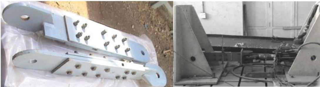
Figure 2-39. Friction dampers on the left and its test setup used for characterization (Kiran et. al., 2016)
