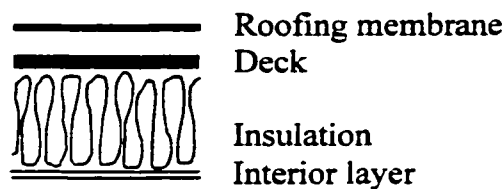
Figure 4.1. Schematic representation of the four basic layers of a light weight flat roof system.
