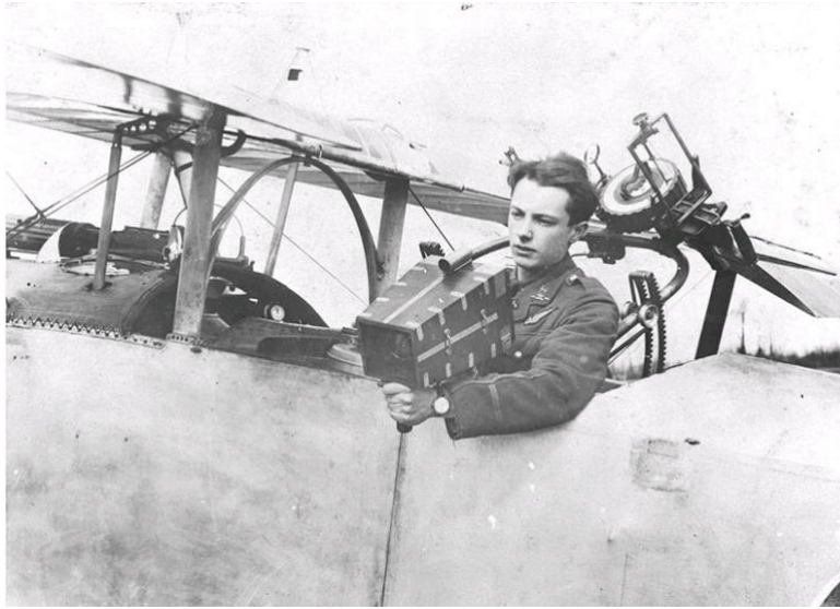
Fig. 5) Lieutenant SC Thynne demonstrates the use of a hand-held camera in the Back seat of a Nieuport aircraft. Example of an A-type camera used during WWI. (UK National Archives)
