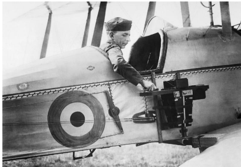
Fig.6) An observer of the Royal Flying Corps in a Royal Aircraft Factory B.E.2c reconnaissance aircraft demonstrates a C type aerial reconnaissance camera fixed to the side of the fuselage, 1916. (UK National Archives)
