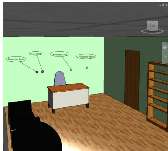
Figure 6-3: Visualization of sensors in 2D and 3D views in the BIM model
