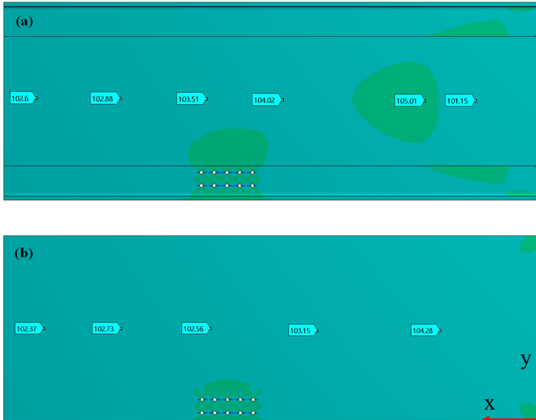
Figure 31 – Static analysis spar (a), web (b). Normal stress along the loading direction at different locations are shown for verification purposes.
