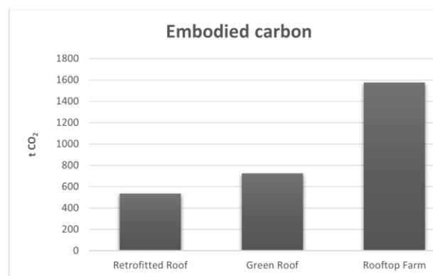
Figure 6.12 Green roof and rooftop farm embodied carbon.
