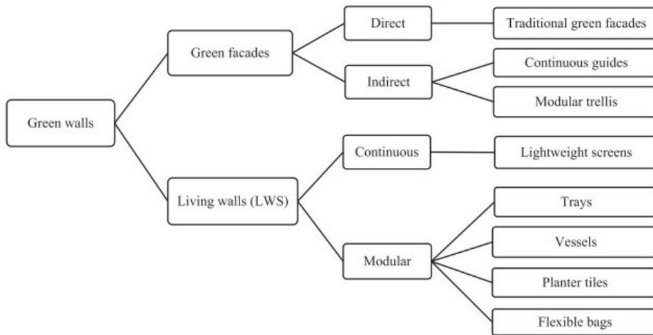
Figure 3.13 Classification of green walls, according to their construction characteristics.[13]
