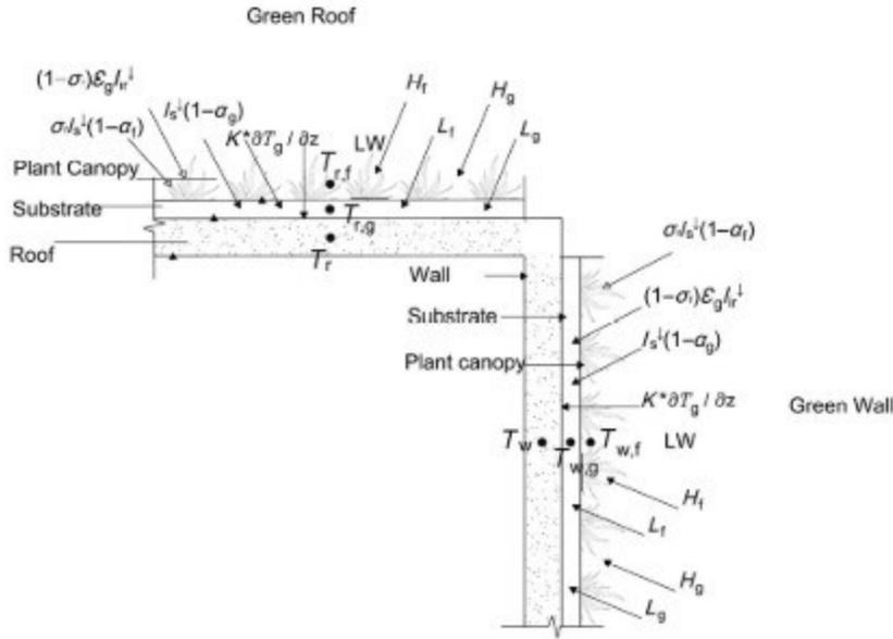
Figure 3.15 Heat fluxes in green roof and green wall based on the EnergyPlus mathematical model[14].
