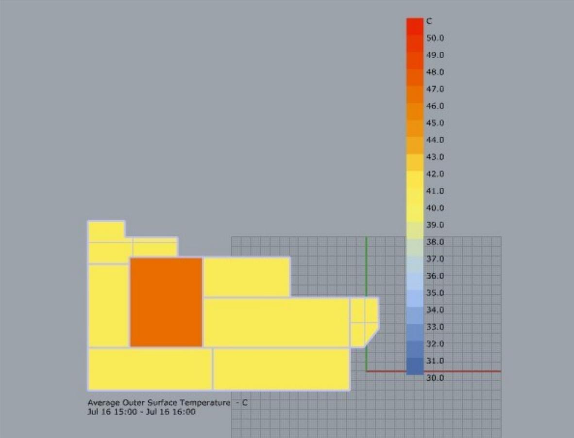
Figure 6.13 Extensive Green Roof and concrete surface temperate comparison
