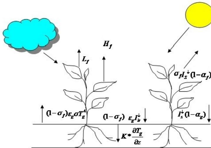
Figure 4.2 The Energy Balance for a Green Roof [17]
