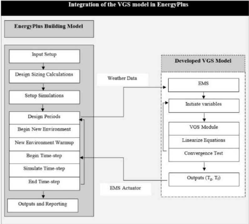
Figure 3.16. Integration of VGS Module with EnergyPlus using features of EMS[15].
