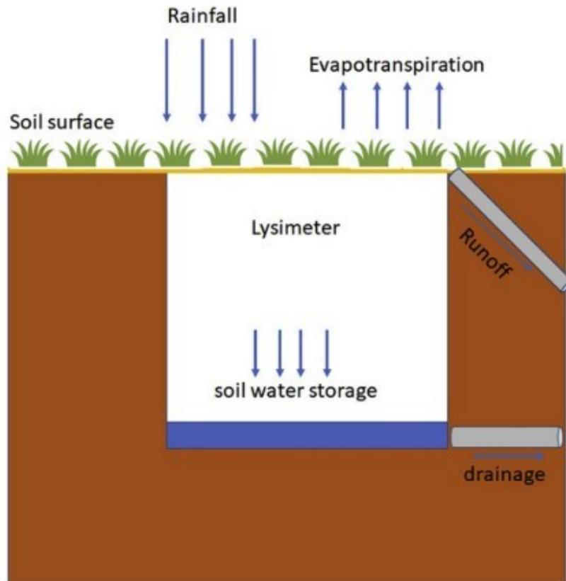
Figure 4.4 Schematic representation of the soil water balance in weighing lysimeter.
