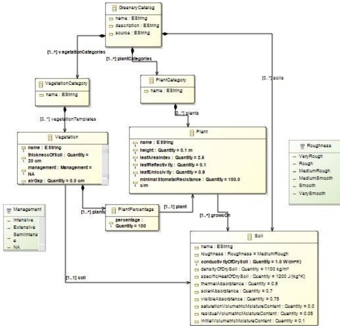
Figure 5.1 Greenery System UML diagram
