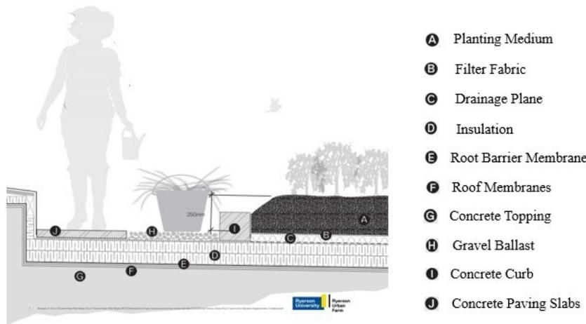
Figure 3.10 Ryerson Urban Farm construction layers
