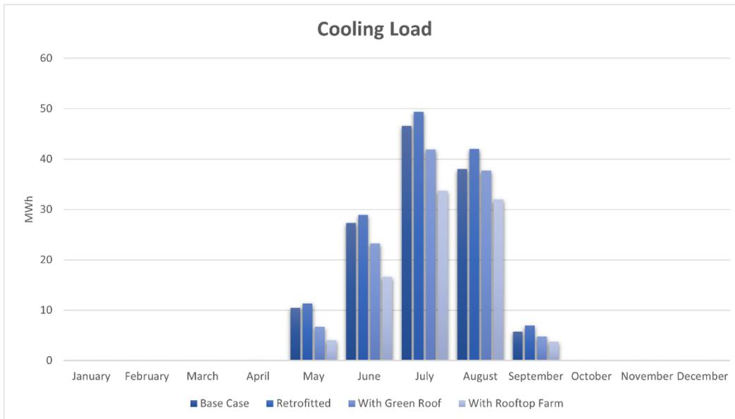
Figure 6.11 Monthly Cooling Load for Base, retrofitted case, and GR Scenarios.
