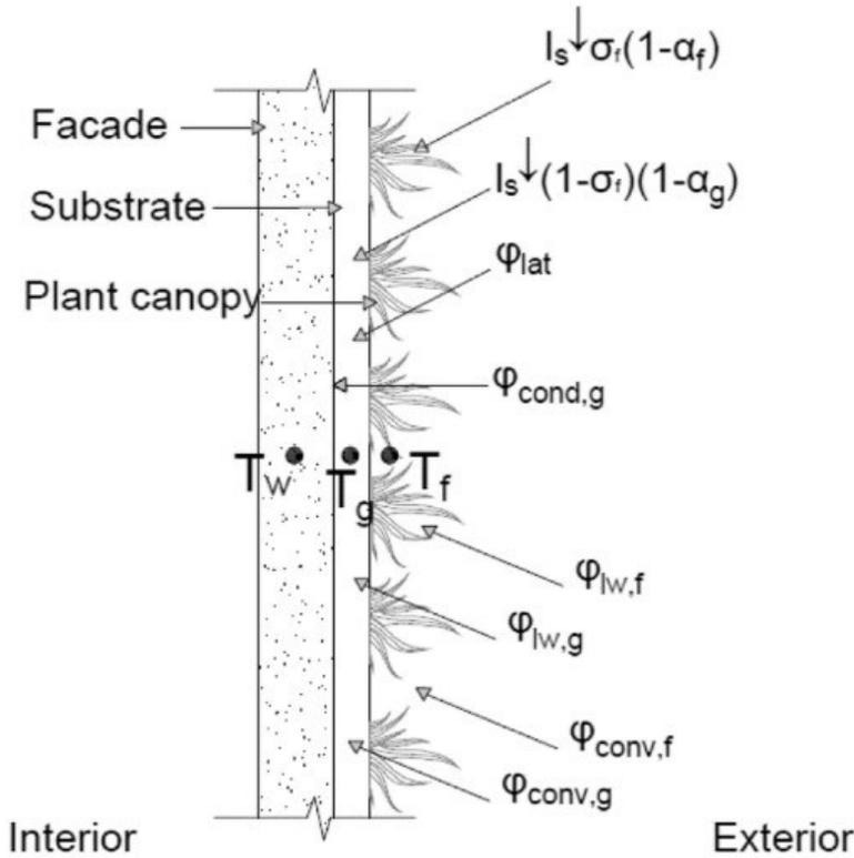
Figure4.3 Heat Fluxes account in the proposed Green wall model[15].
