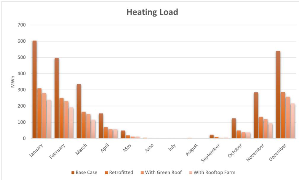
Figure 6.10 Monthly Heating Load for Base, retrofitted case, and GR Scenarios.
