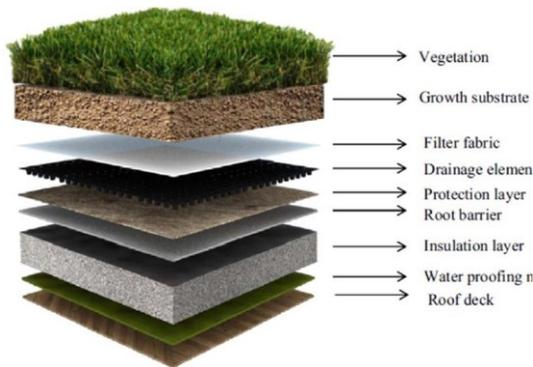
Figure 3.6 Schematics of different green roof components[9]
