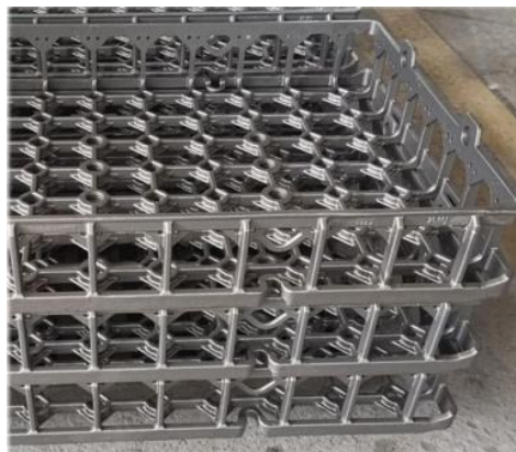
Figure 1.2 Heat Treatment Rack (Eternal Bliss Casting & Forging Co., LTD)
