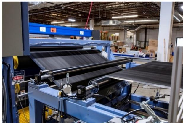
*Figure 3.1: 60"-wide ZRT film production line installed at Boston Materials' factory in Billerica MA, USA [26]*
