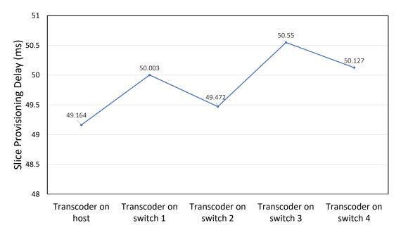
Figure 5.7: Slice provisioning delay for different scenarios.
