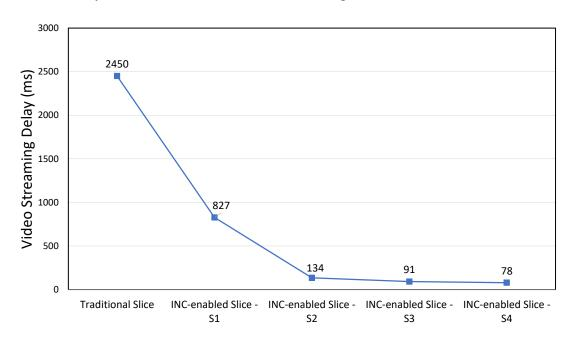
Figure 5.6: Video streaming delay for traditional slice vs. INC-enabled slices in different scenarios.
