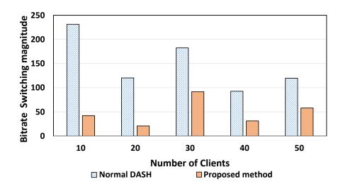
Figure 3.5: Bitrate switching in two DASH methods for five set of clients.
