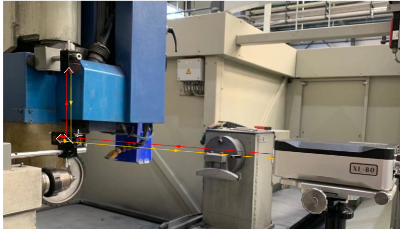
Figure 4.12 Geometric errors of the linear axes were identified with a laser interferometer
