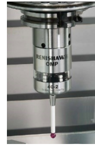
Figure 1.1 (a) On-machine tool setters and (b) an on-machine touch triggered probe.
