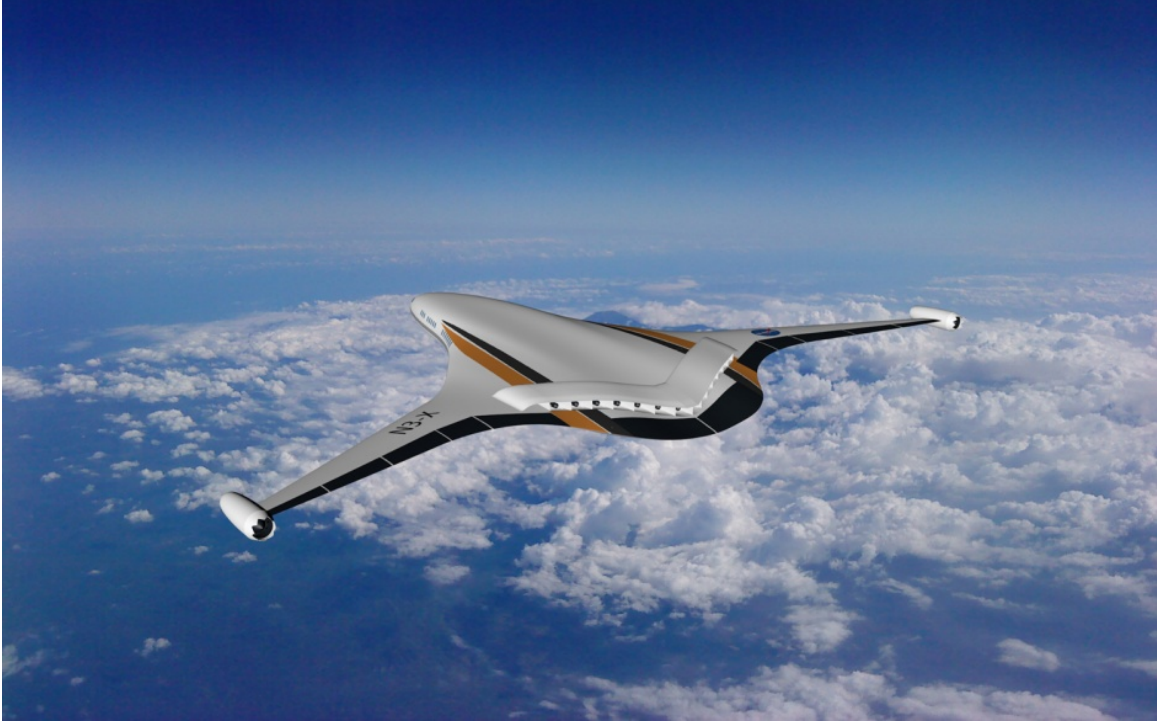
Figure 1.2. NASA N3-X blended wing body aircraft concept with turbo-electric distributed propulsion system [3].
