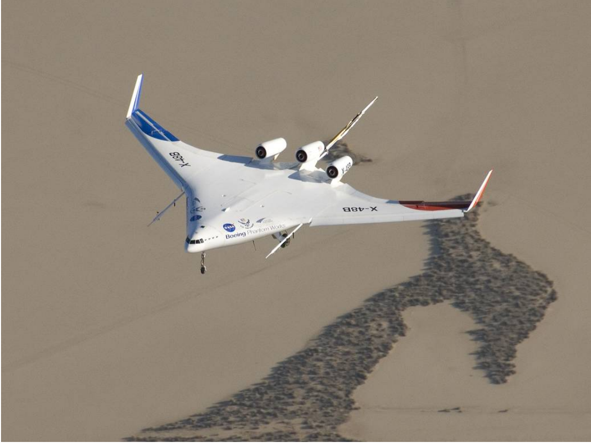
Figure 1.1. Boeing’s sub-scale X-48B blended wing body aircraft without distributed propulsion flew over the edge of Rogers Dry Lake at Edwards Air Force Base during its fifth flight on Aug. 14, 2007 [2].
