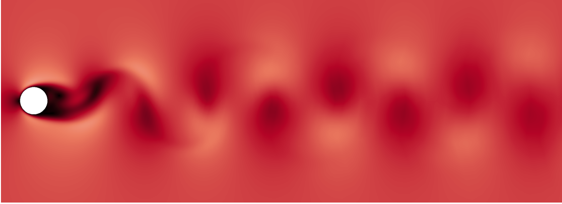
(b) Velocity field for K = 3 for Mesh 1.
