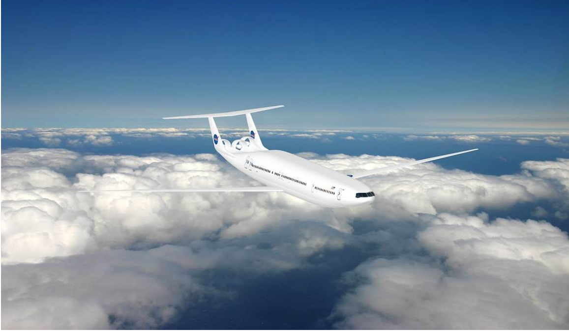
Figure 1.3. The double bubble D8 aircraft concept with engines flush mounted on the top rear of the fuselage, designed based on a concept known as Boundary Layer Ingestion (BLI), claimed to achieve a 36% reduction in fuel burn from its configuration [4]. This aircraft is designed to fly at Mach 0.74 and carry 180 passenger for domestic flights [5].
