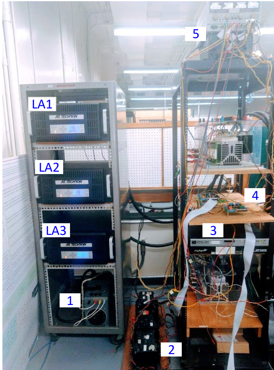
Fig. 2.23. LA1, LA2, LA3 – three-phase Linear Amplifiers, 1- three-phase variac, 2 - link filters, 3 - Opal-Rt, 4 - protection circuit and sensors, 5 - DC power supply.
