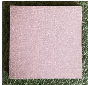
Figure 4.3. Images of samples 10-18 (grit-blasted under the pressure of 80 psi) in comparison to the as-fabricated state utilized for visual inspection.
