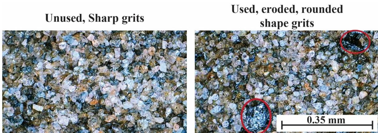
Figure 4.24. Digital microscope images of the unused and used grits.
