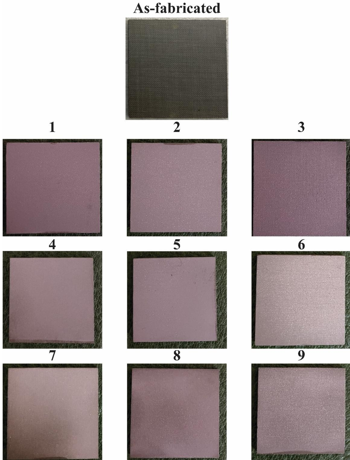
Figure 4.2. Images of samples 1-9 (grit-blasted under the pressure of 60 psi) in comparison to the as-fabricated state utilized for visual inspection.
