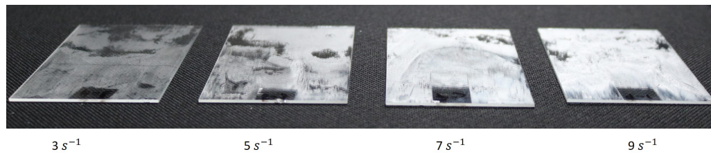
Figure B.3: Holes observed on glass substrate. Their size and frequency decreases with shear rate.
