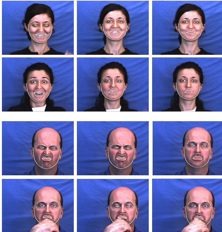
Figure 5.5: Examples of facial landmarks detected using dlib toolbox from faces for different emotions. First row: Happiness. Second row: Positive Surprise. Third row: Anger. Fourth row: Puzzlement.
