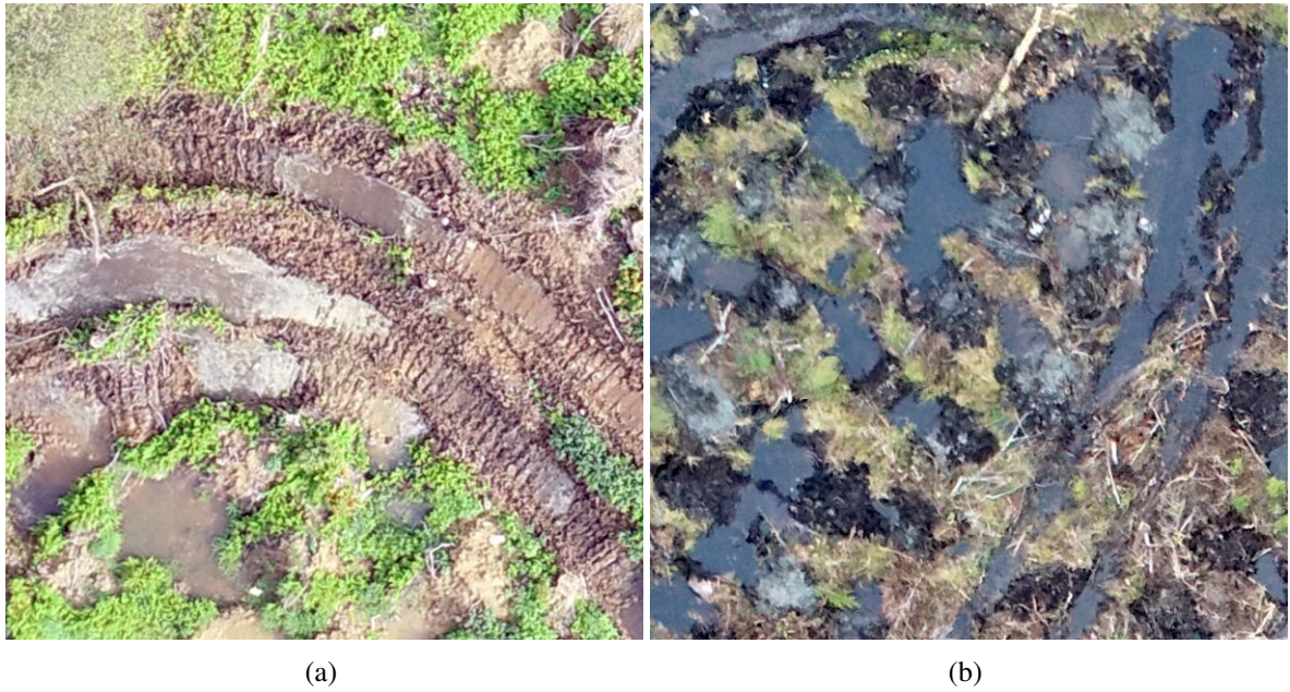
Figure 4.5: Illustrations of destroyed mounds. (a) Mounds that were destroyed during mechanical preparation by the excavator. (b) Mound destruction due to heavy rain.
