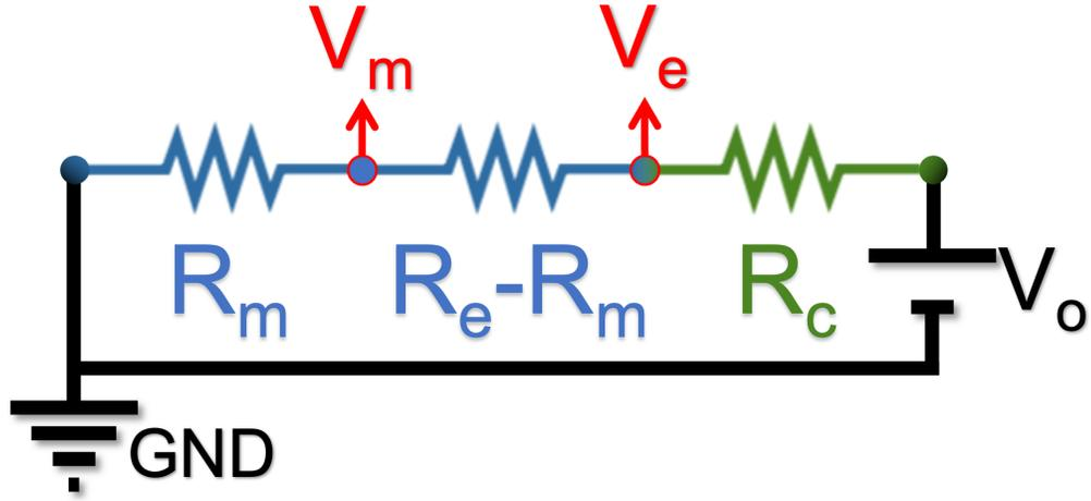
Figure 4.7: Detailed equivalent electrical model of the sensing element with the placement of electrode voltage measurements.
