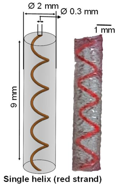
Figure 1.7: PDMS pillars with 3D microfluidic channels inside [40].
