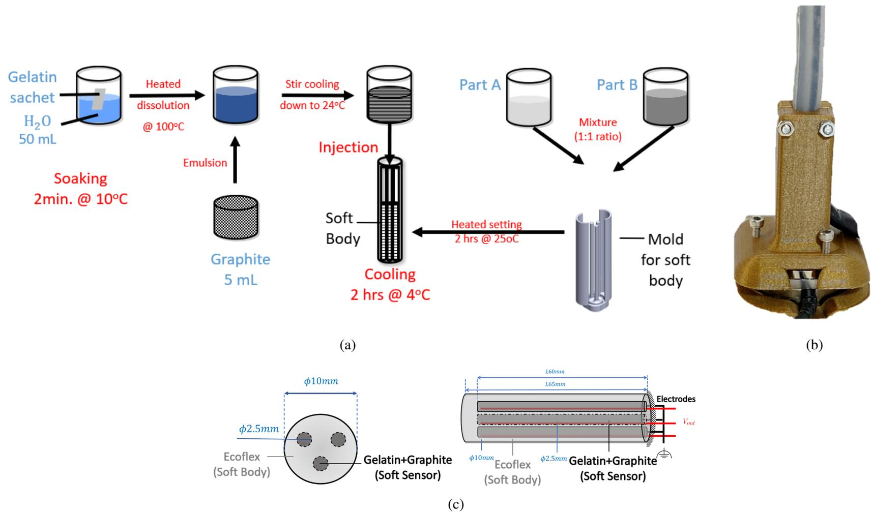
Figure 3.2: (a) Schematic process flow of fabricating the sensing element, i.e., gelatin-graphite composite., (b) prototyped sensor embedded in a soft flexure, and (c) geometric design of the sensor and flexure.
