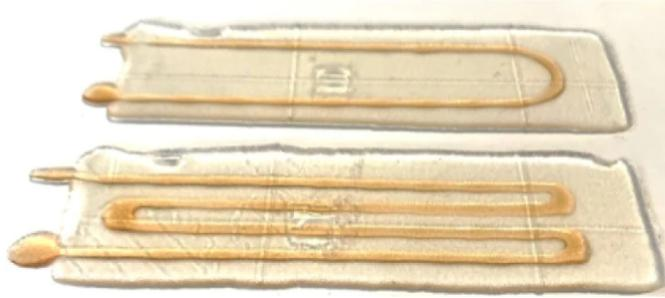
Figure 1.9: Self-healing ionic gelatin/glycerol hydrogel strain sensor [63]
