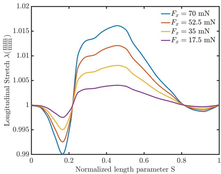
Figure 4.5: Variation of stretch along the sensing element in three simulation loadings.
