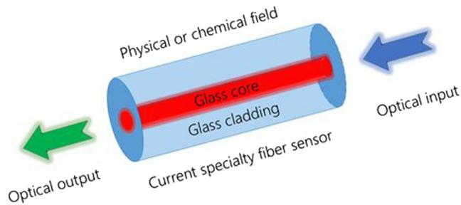
Figure 1.3: Traditional specialty optical fiber sensor schematic [17]
