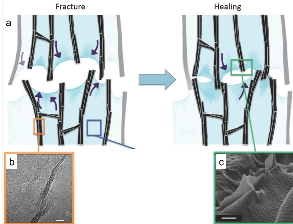
Figure 1.10: a) A diagram of the healing procedure. b) The network walls consist of intertwined graphene flakes (transmission electron micrograph). d) Fracture exposes the carbon network walls (scanning electron micrograph of a fracture surface). Capillary forces caused by polymer flow bring the wall together, re-establishing the link between the network's walls, while the polymer's reversible bonds allow for complete matrix repair [86].
