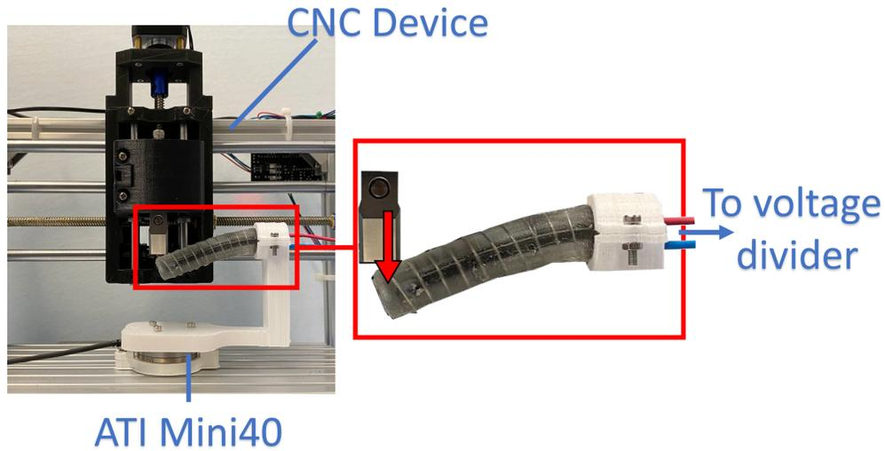
Figure 2.5: Test setup for experimental validation.
