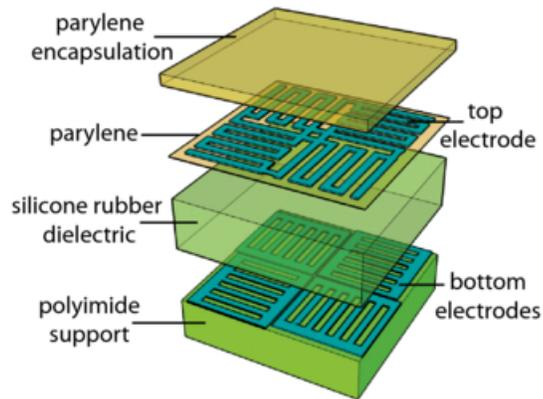
Figure 1.5: Two layers of metallic electrodes are placed in three layers of polymeric packaging to form a flexible capacitive force sensor [27].
