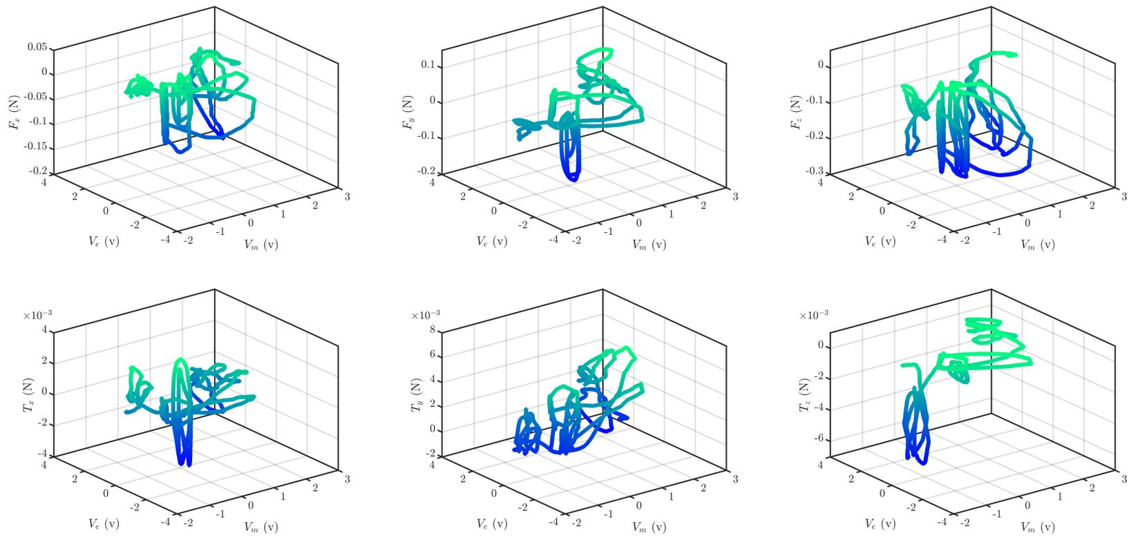
Figure 4.11: Feature-space visualization of the training output used for nonlinear calibration, (a–c) force output and (d–f) torque output.
