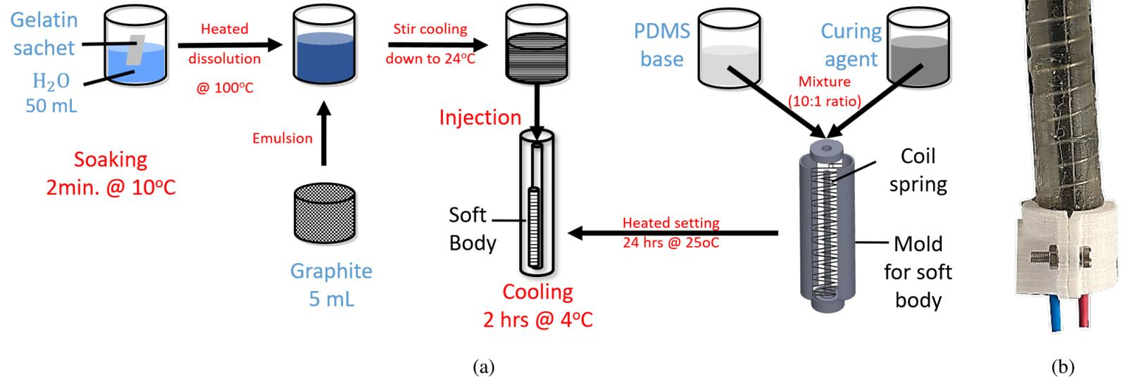
Figure 2.2: Fabrication of gelatin and graphite mixture inside PDMS layer.
