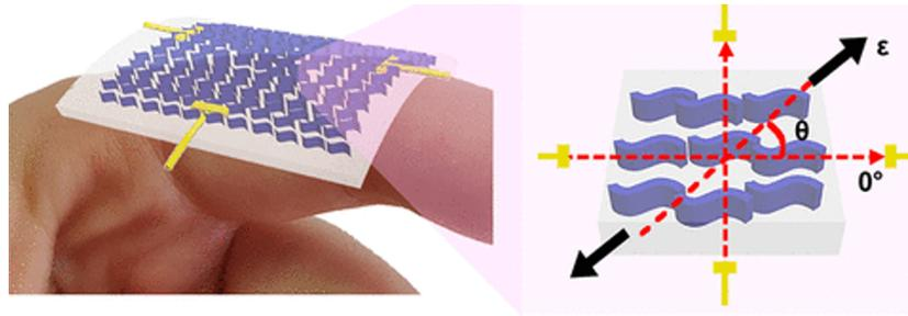
Figure 1.11: Stretchable strain vector sensor capable of concurrently detecting strain directions and amplitudes [89].
