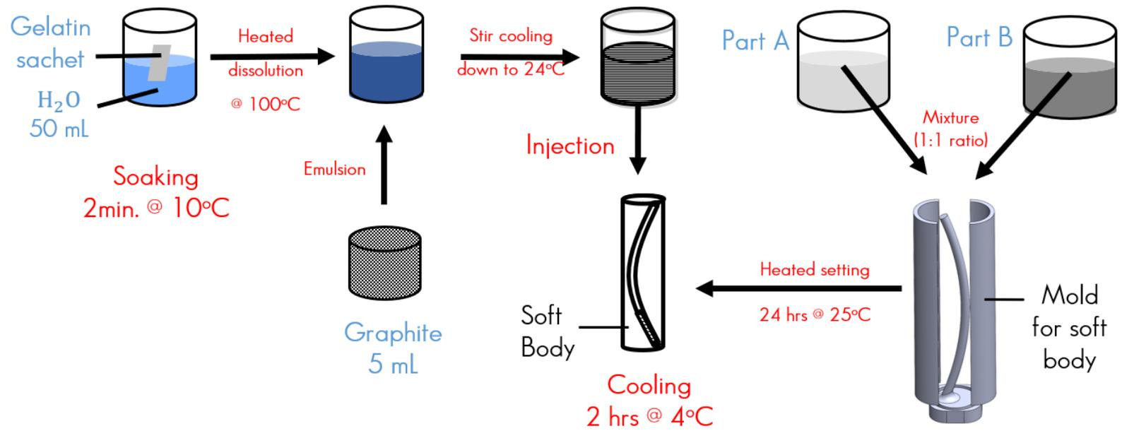
Figure 4.3: Fabrication of gelatin and graphite mixture inside Ecoflex layer.
