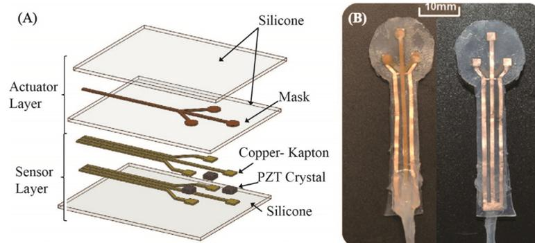
Figure 1.6: the schematic of the multi-layer construction of piezoelectric soft skin [28].
