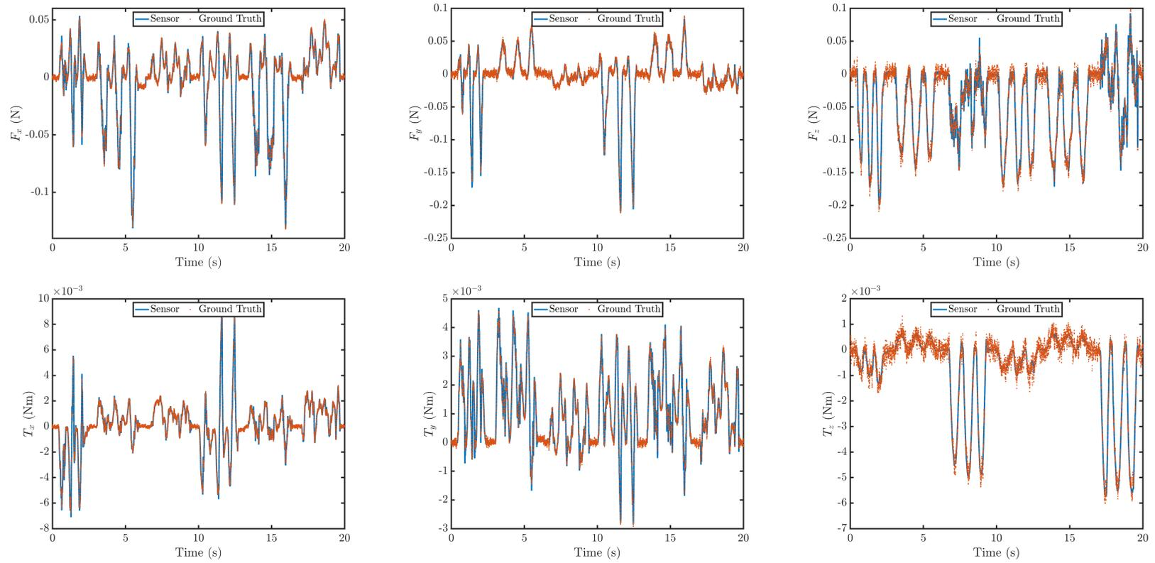
Figure 4.13: Comparison of forces and torques estimated by the proposed sensor versus ground truth.
