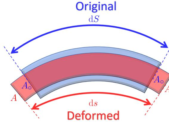
Figure 2.3: Differential element of the sensing element under deformation.
