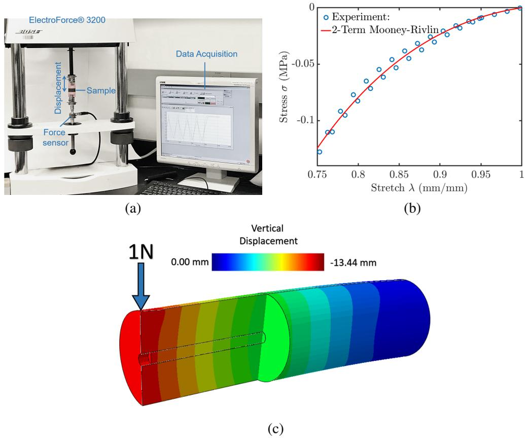
Figure 2.4: (a) Setup and a representative sample under compression test, (b) a stress-stretch diagram for the PDMS sample, and (c) deformation of the finite element model.
