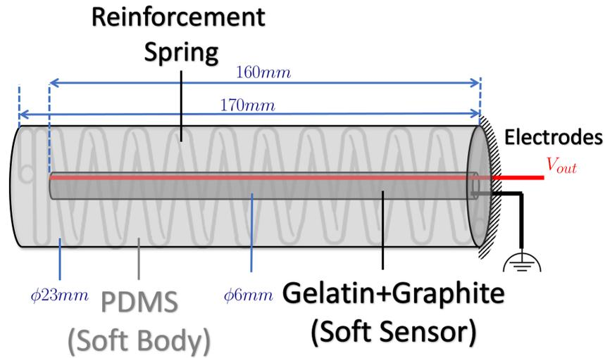
Figure 2.1: The structural design of the sensor with gelatin/graphite capsulated inside PDMS.
