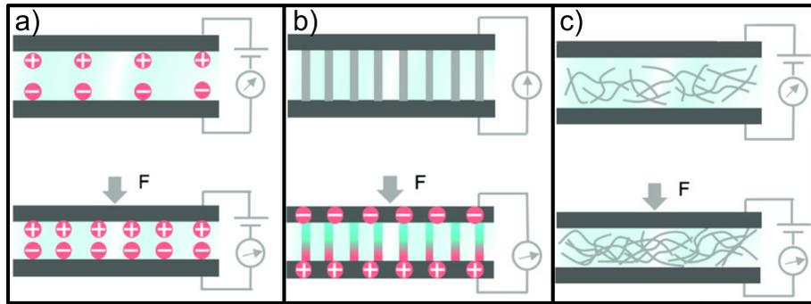
Figure 1.4: Electric sensors' sensing concept a) Capacitive, b) Piezoelectric, and c) Piezoresistive [23].
