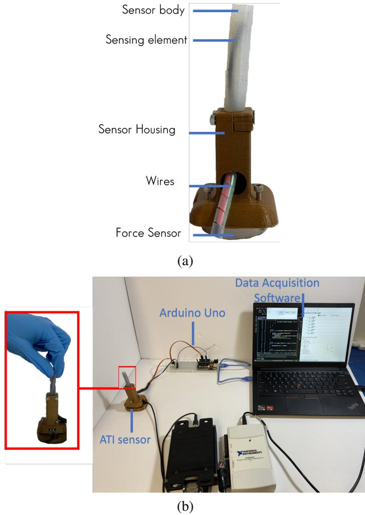
Figure 4.9: (a) Sensor prototype, (b) Experimental setup for calibration and validation tests.
