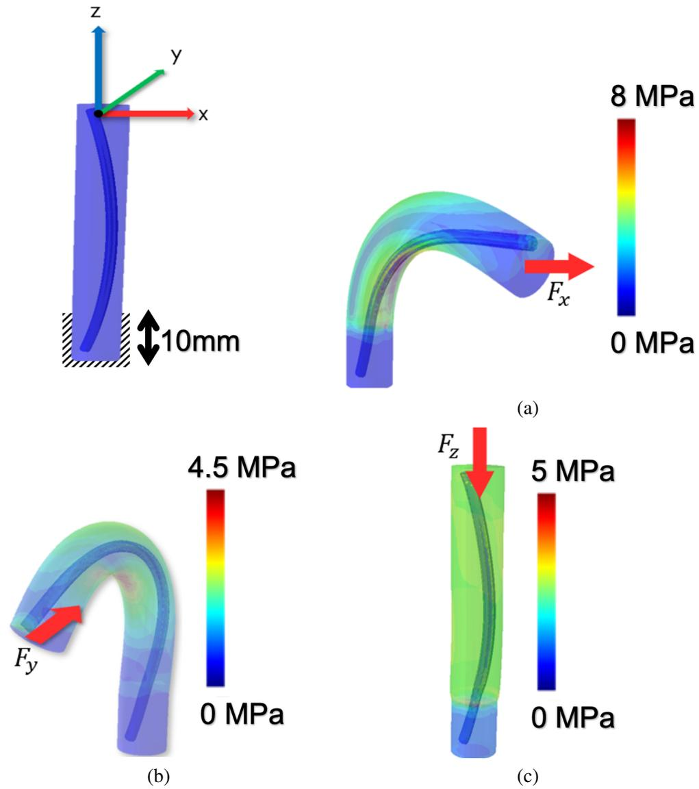
Figure 4.6: Von Mises stress contour of the finite element model for (a)  $F_x = 70$  mN. (b)  $F_y = 40$  mN, and (c)  $F_z = 70$  mN.
