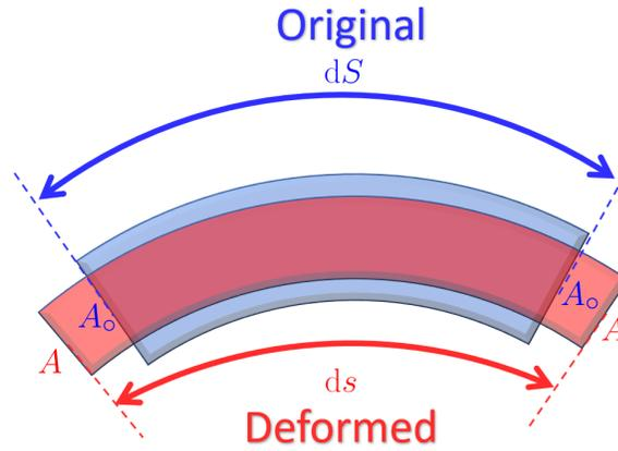
Figure 4.4: Differential element of the sensing element under deformation.
