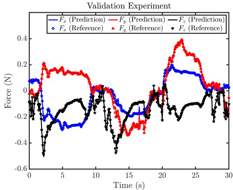
Figure 3.5: Comparison of predicted and reference force components in the validation test.
