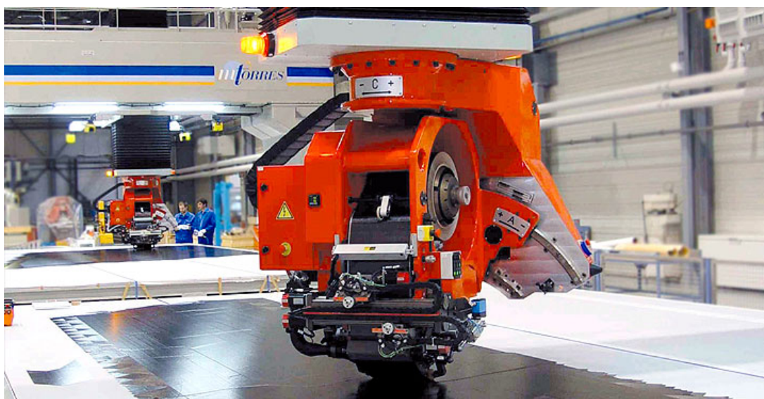
Figure 2.3: Automated Tape Layup (Photo credit: mtorres) [19]
