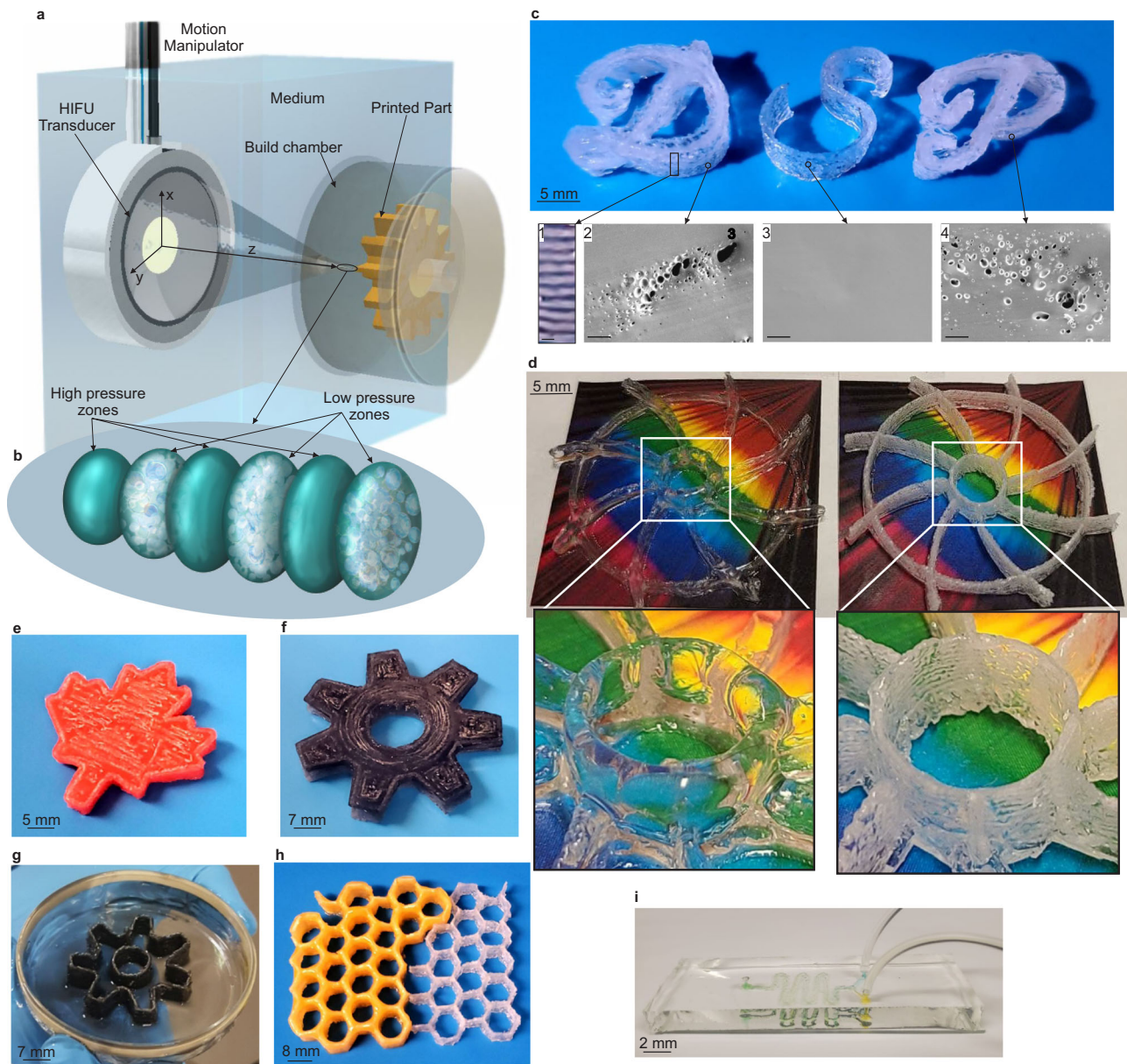
Fig. 1 DSP concept and printed parts. a DSP process schematic. b Detailed view of UAMR, bubbles are created in low-pressure zones. c Printed “DSP” letters. c1 porous/transparent structure of the printed part (the scale bar is 200 \mu\text{m} ). c2–4 , SEM pictures of the microstructure of the printed parts (the scale bar is 100 \mu\text{m} ). d Printed impellers, transparent and porous. e–h Printed maple leaf, gear, shell and honey comb, respectively. i Molded microfluidic channel using 3D printed PDMS mold. (HIFU: high-intensity ultrasound).
