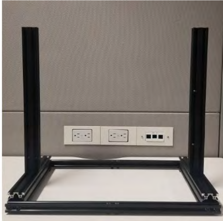
Figure A.28: Rear Horizontal Extrusion install.
