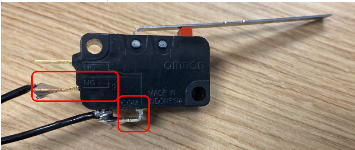
Figure A.10: Pump Limit Switch soldering.
