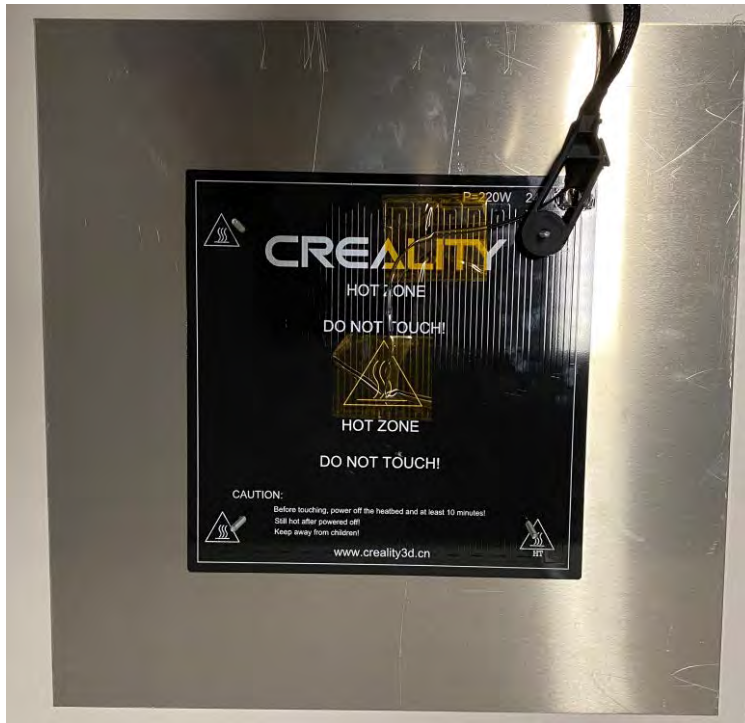
Figure A.39: Heated Bed placement over Ender Xtender Platform.
