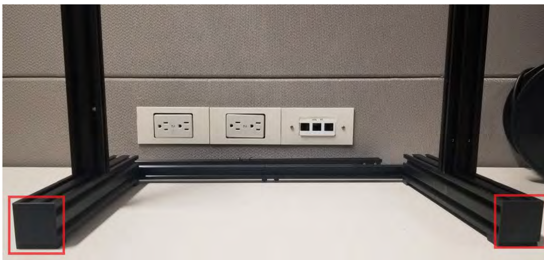
Figure A.27: Rear frame extrusion cover removal.
