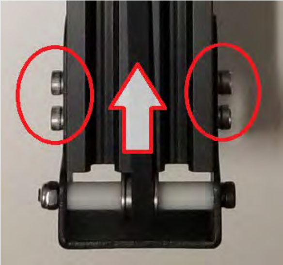
Figure A.15: Y-Axis Belt Tensioner removal.
