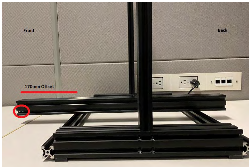
Figure A.30: Y-Axis Extrusion alignment.
