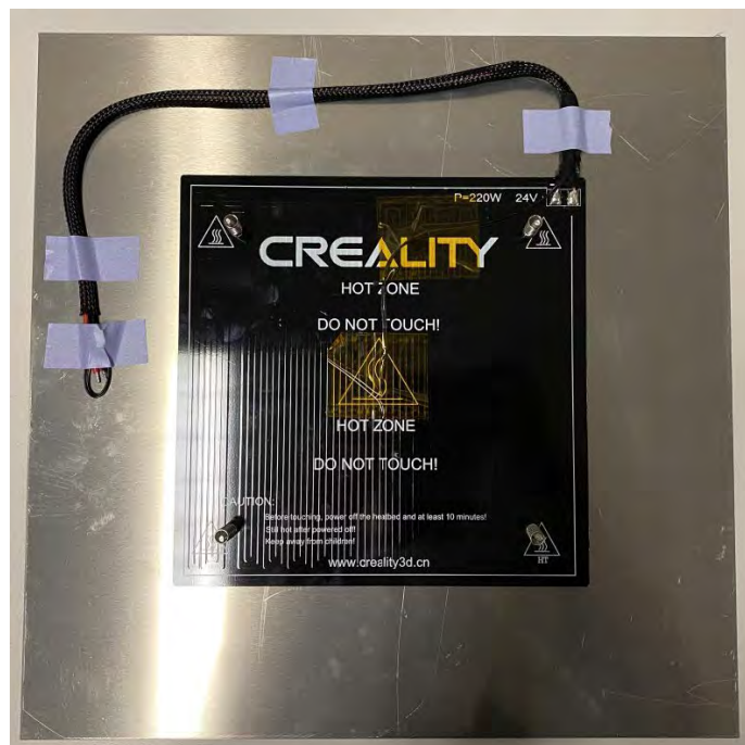
Figure A.42: Heated Bed attachment to Ender Xtender Platform.
