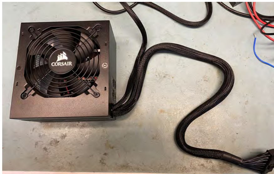
Figure A.55: 450W modular ATX PC power supply.
