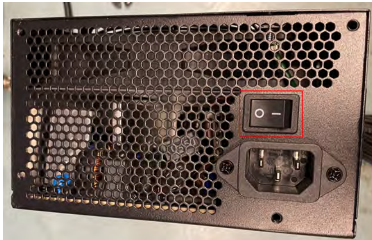
Figure A.54: Always ensure the power supply is OFF when cutting or soldering the wires.
