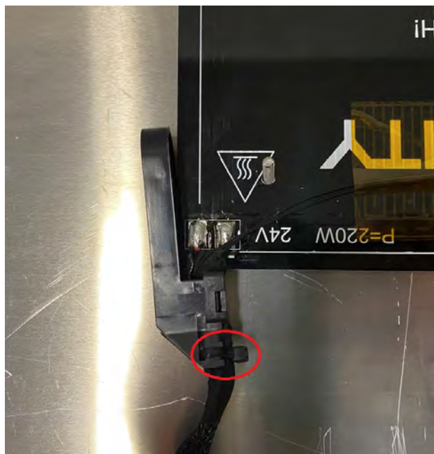
Figure A.40: Removing plastic part from Heated Bed wires.
