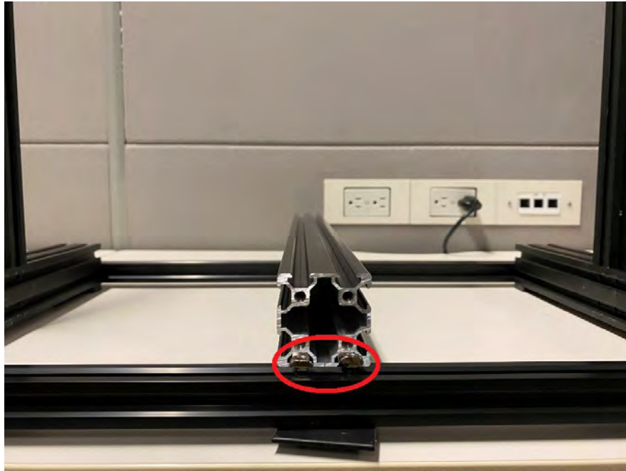
Figure A.29: Y-Axis Extrusion install.
