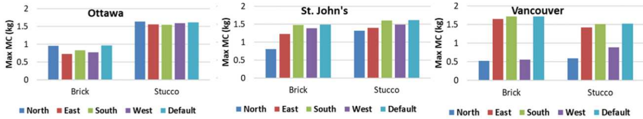
Figure 3.9: Maximum Moisture content of OSB layer for three cities with WDR but no water source
