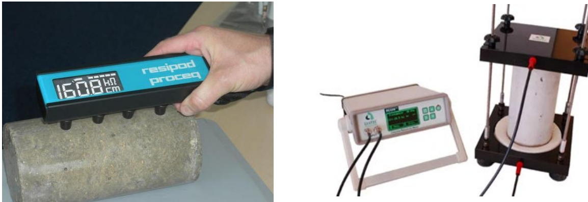
Figure 7: Surface resistivity test device (Proceq's Resipod (left) and Giatec surf TM (right)).
