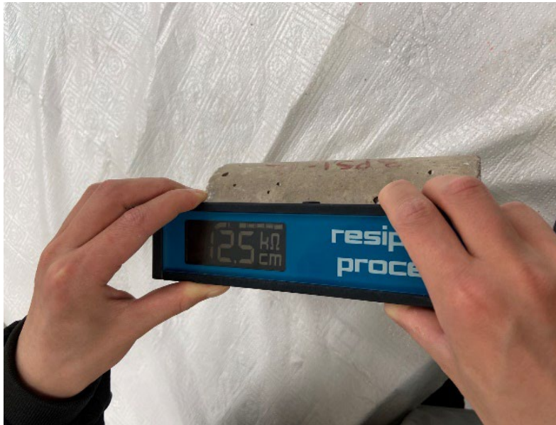
Figure 24: Testing the surface resistivity.
