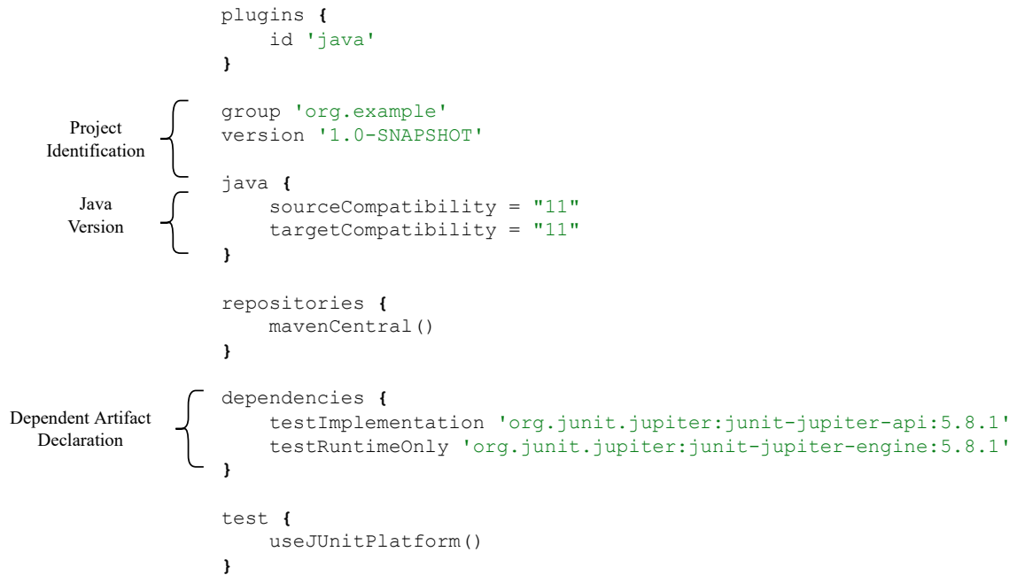
Figure 3.3: Gradle Build File
