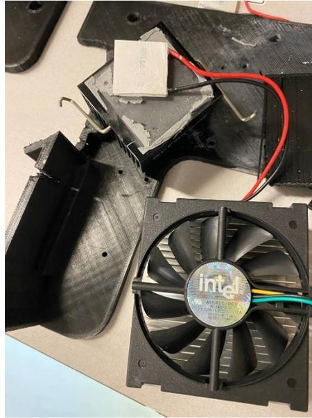
Figure 3-19 Peltier, Fan, and heat sink
