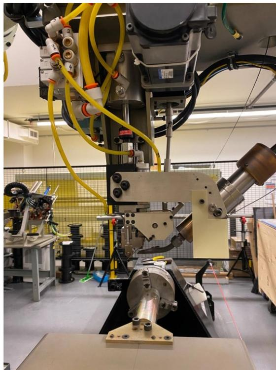
Figure 1-6 Thermoplastic AFP head at Concordia University
