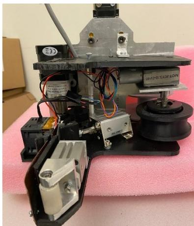
Figure 3-35 View of the bottom side of the AFP head
