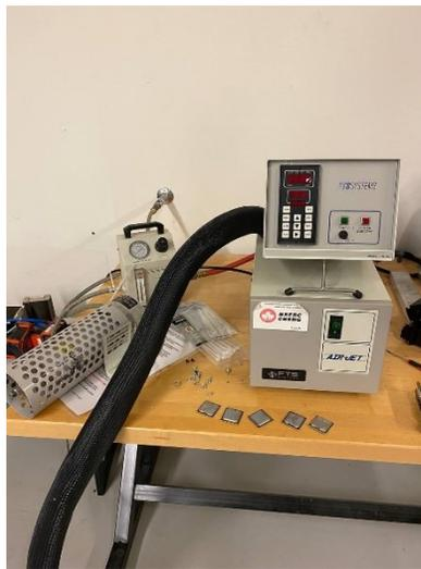
Figure 3-18 Air jet system
