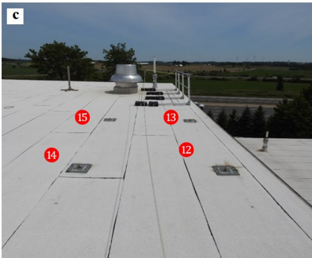
Figure 2: Photos of pressure taps on the lower and upper roofs
