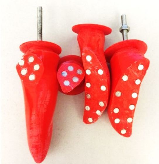
Figure 3.11 LV and RV molds with the placed magnets
