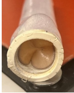
Figure 3.14 Aortic valve sutured to the silicone aorta
